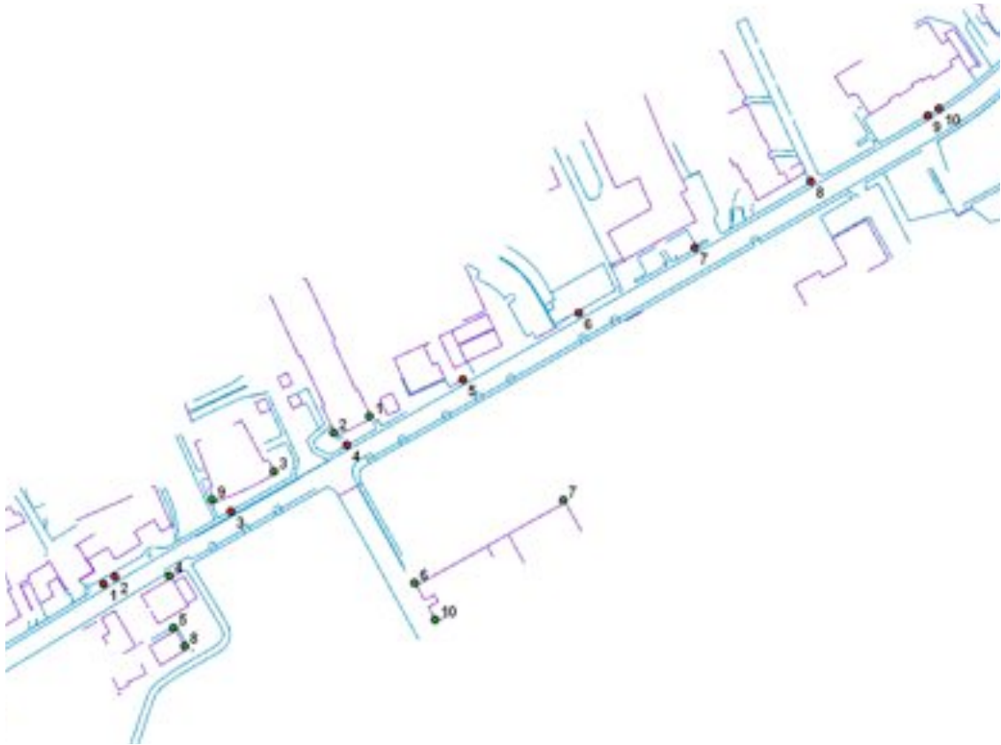
Figure 3.6: GIS information about a street. Purple represents building outlines. Blue shows curbstones.
