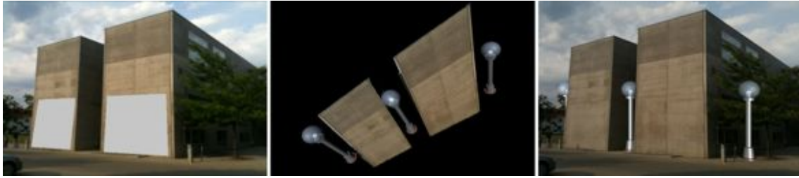
Figure 5.5: Combining sparse information with image coherence. (Left) Sparse GIS model data overlaid over a registered view. (Middle) Segmentation of the registered view derived from the sparse model. (Right) Correct occlusion with virtual geometry using the derived depth map.
