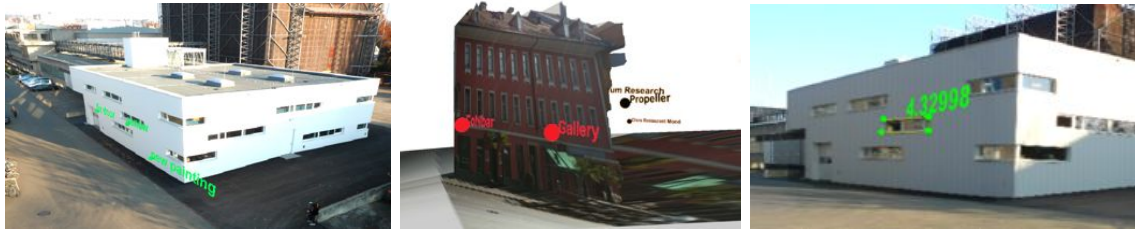
Figure 5.18: Using the dense depth maps in other AR applications: (Left) Annotating a building. The dense depth map allows to make annotations spatially consistent. (Middle) Labeling. The dense depth maps helps to filter visible labels (marked red) from invisible (marked black). (Right) Surveying. The user can interactively survey parts of the building by using the dense depth map as interaction surface.
