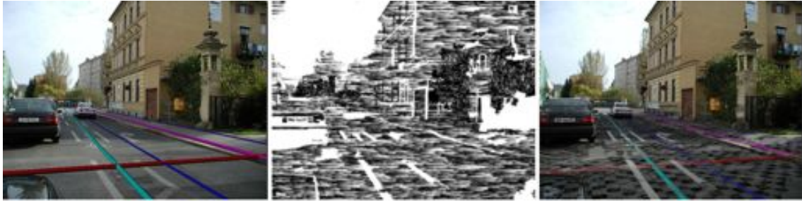
Figure 4.2: Image-based ghostings. Left) Naïve overlay of virtual pipes on top of a video image of an urban scene. Middle) Extracted important image regions. Right) Ghosting preserves important image parts in the final rendering and provides a convincing integration of the virtual pipes into the street scene.
