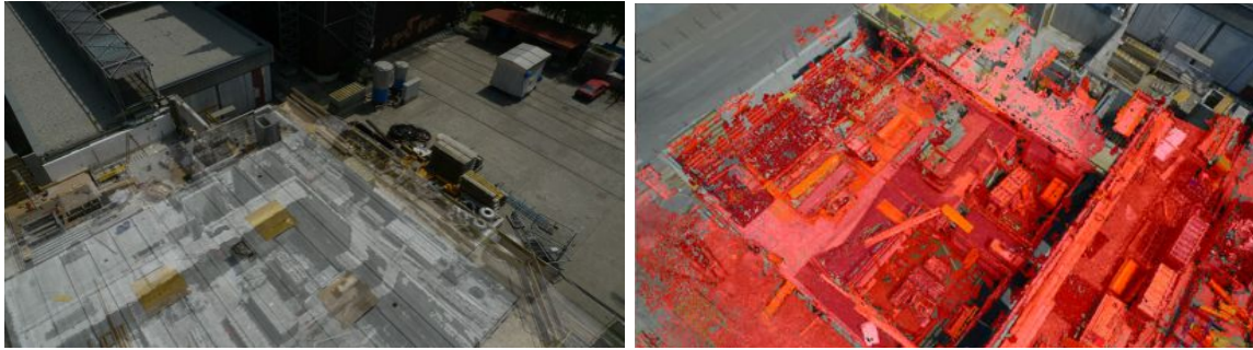
Figure 7.1: Simple blending of complex data. The current state of the construction site is overlaid with 3D data of one previous point in time. Left) Transparent overlay. Right) Overlaying a colored point cloud for highlighting the difference between virtual data and physical environment.
