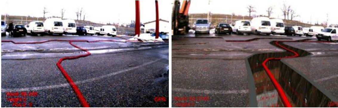
Figure 1.8: Adding virtual pictorial cues to an X-Ray visualization: (Left) The virtual object is visualized in the X-Ray AR view without additional hints. Without additional depth cues it is nearly impossible to judge the depth of the virtual object in relation to the physical ground. (Right) By rendering a virtual excavation along the virtual object, additional depth cues are provided.
