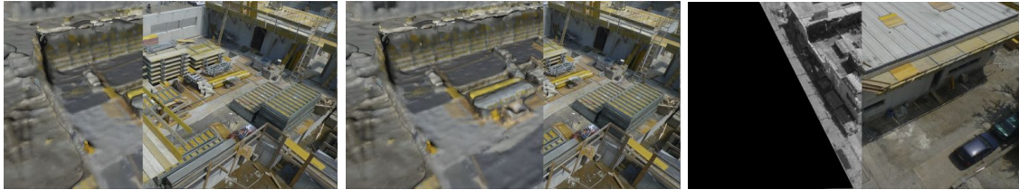
Figure 7.3: Side-by-side visualization using 2D sliders. The mouse input defines the border between video image and virtual content. Left and Middle) The virtual content is overlaid on the right side of the border. Right) On the right side of the border only the virtual data representing a previous point in time is displayed.
