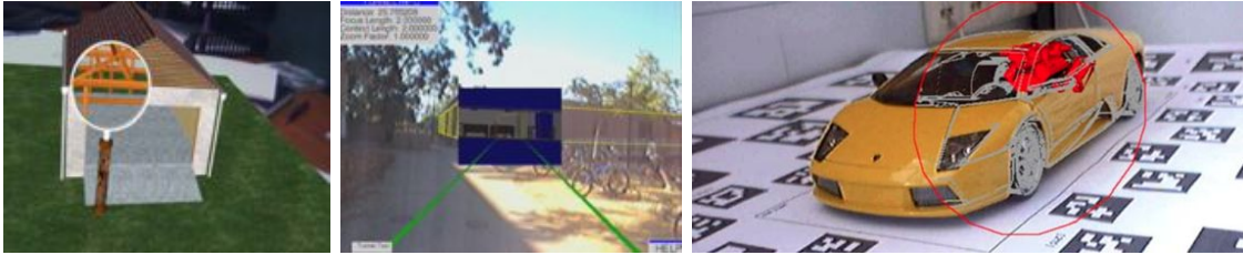
Figure 2.17: Focus&Context techniques for information filtering in AR. Left) Magic lens that defines a focus area for displaying defined virtual content [76]. Middle) Interactive X-Ray tunnel [8]. Right) Focus&Context allows to explorer occluded information in an X-Ray view [54].
