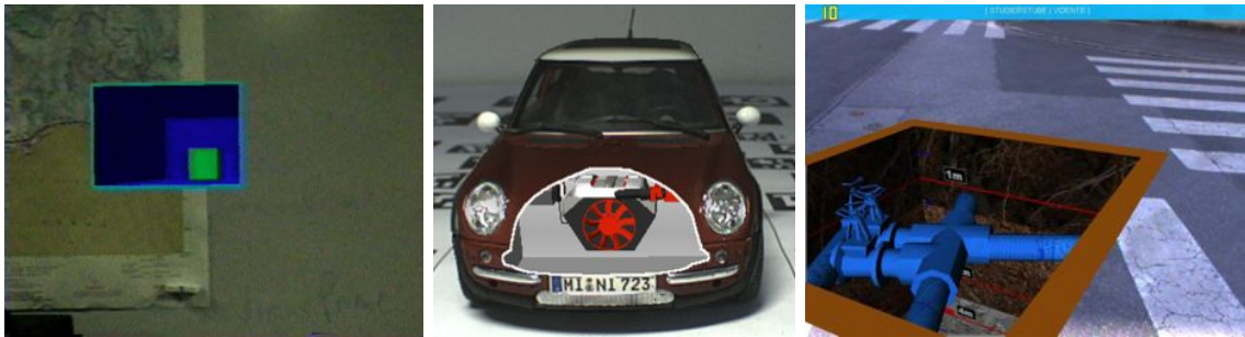
Figure 2.15: Cutaways as virtual cues in AR. Left) Virtual cutaways rendered on a wall to reveal a hidden green target object. Middle) Virtual cutaways used to visualize the interior of a car [53]. Right) A virtual excavation with a depth scale is used to visualize subsurface infrastructure in an urban civil engineering scenario [78].
