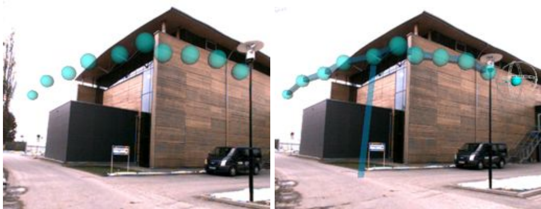
Figure 6.6: Visualization techniques for virtual floating objects. Left) Visualization without virtual depth cues. Right) Visualization with depth cues for floating objects.
