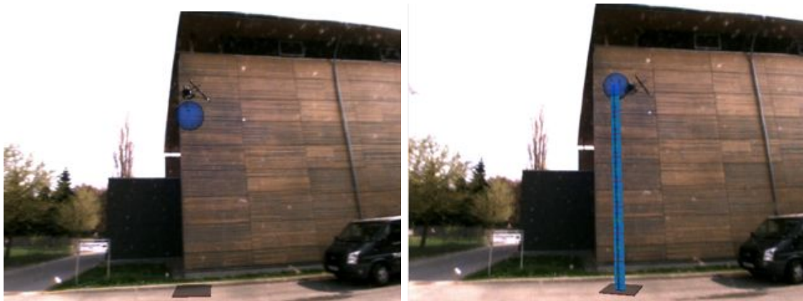
Figure 6.5: Additional graphical hints for supporting the understanding of the position of the MAV (Asctec Falcon 8 in black). Left) Sphere representation of the waypoint and its shadow projection on the ground. Right) Connection line combined with shadow.
