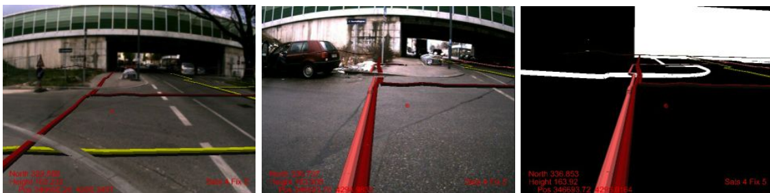
Figure 5.2: Using sparse data for occlusion culling. (Right and Middle) Hidden virtual information that is located under the curbstones is culled from the rendering to preserve the physical information of the curbstones. (Left) For this purpose we create a mask based on the virtual representation of physical objects of interests.
