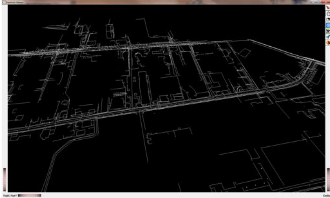
Figure 3.7: Semantic scenegraph representation. Each VidenteGML feature is converted into a 3D scenegraph object. The scenegraph object includes the geometric properties, but maintain the semantic information as well.
