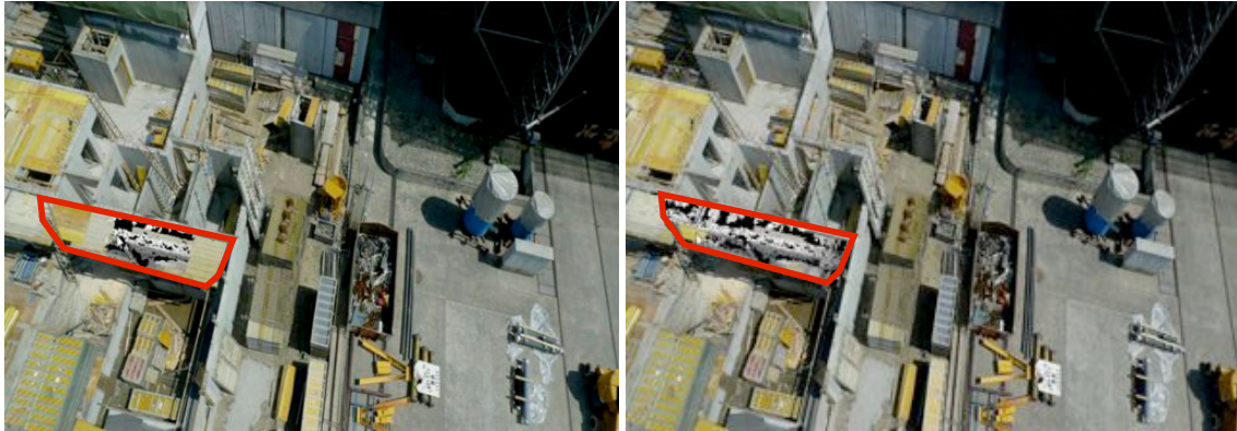
Figure 7.5: Information Filtering by selecting 2D image regions. The user interactively selects image regions in the AR view. For the selected regions the virtual information is displayed (highlighted in red).
