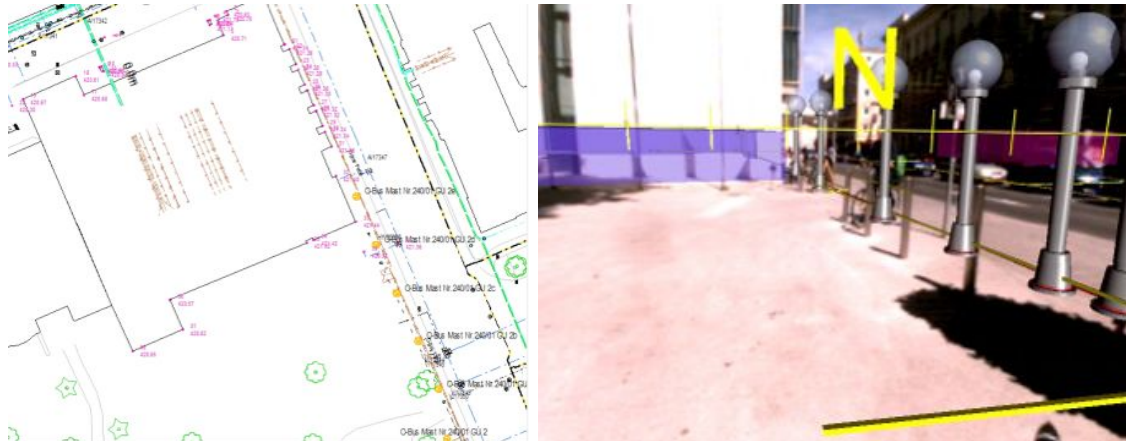
Figure 2.20: Traditional paper plans vs. an AR interface for planning. Left) Paper-based planning, newly planning lamps are visualized in orange. Right) AR interface for planning lamps.
