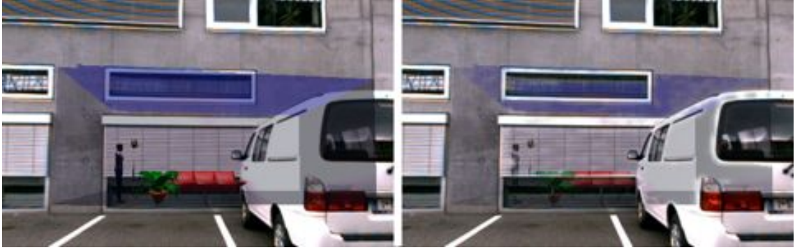
Figure 4.5: X-Ray visualization of a virtual room inside a building. The left image shows the simple overlay, where the room is more perceived to be located in front of the building. The right image shows the usage of image-based ghostings. Occlusion cues are extracted from the video image and preserved in the visualization. The virtual room is perceived to be located inside the building.
