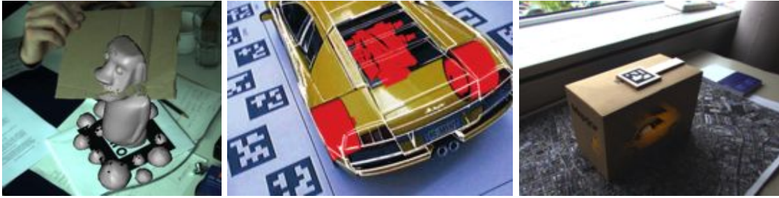
Figure 2.9: Examples for using model-based physical cues. Left) Using time-of-flight camera data for occlusion culling (Courtesy of Fischer et al. [31]). Middle) A ghostings based on edges extracted from a registered 3D CAD model (Courtesy of Kalkofen et al. [55]). Right) Using importance maps applied on a 3D model (Courtesy of Mendez et al. [79]).
