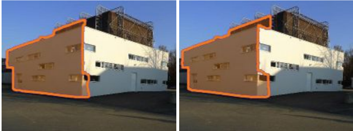
Figure 5.12: Segmentation results for selected offsets. (Left) Segmentation result for 0.5m offset. (Right) The segmentation with an 1m offset shows a larger error but still a visually acceptable result.
