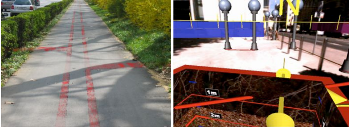
Figure 6.1: Physical depth cues vs. user-centric virtual visual cue. Left) Physical occlusion cues only provide ordinal depth information. Right) A virtual magic lens provides relative depth information.
