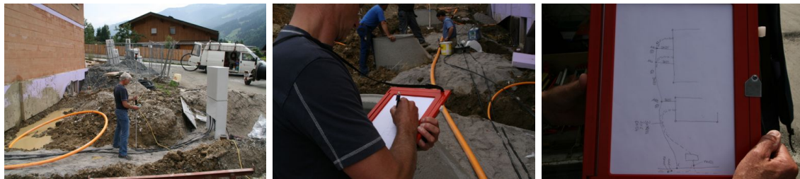
Figure 2.19: Traditional surveying methods. Left) User surveys point of interest using the theodolite. Middle) He has to note down information about the surveyed point (such as type). Right) Overview of a set of surveyed points with additional information.
