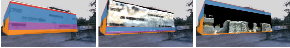
Figure 7.16: Transitions between Visualization Levels with Distorted View. Left: Average Completion Diagram. Middle and Right: By selecting a point in time within the completion diagram the user gets a detailed visualization of the wall at the point in time he selected. To provide still the abstract information, the completion diagram is distorted and presented in the same view.
