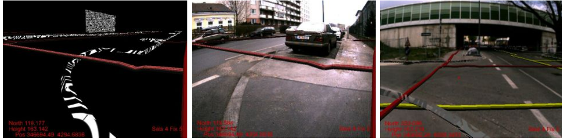
Figure 5.3: Using sparse data in combination with Perlin noise for occlusion culling. (Left) Perlin noise mask mapped to the objects of interest. (Right and Middle) Hidden virtual information that is located under the curbstones are culled from the rendering to preserve the physical information of the curbstones based on the mask.
