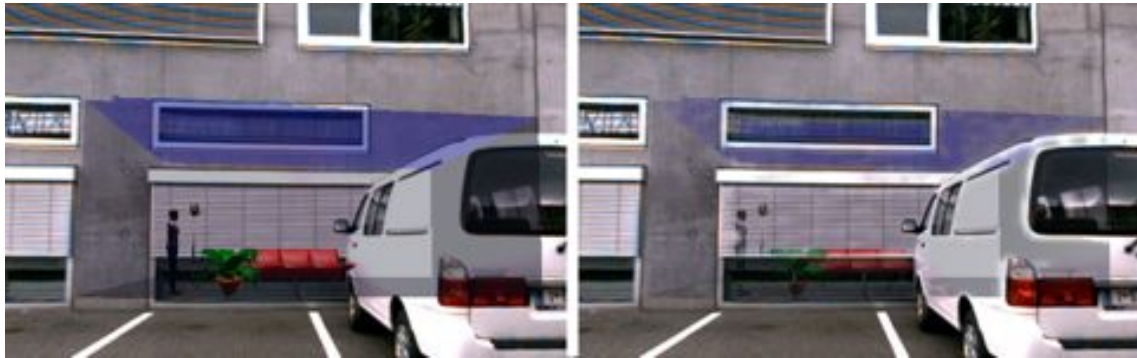
Figure 1.11: Seamless integration of virtual content in an X-Ray visualization of a virtual room inside a physical building. The left image shows a simple overlay, where the room is perceived to be located in front of the building. The right image shows the extraction of occlusion cues from the video image. Occlusion cues are extracted from the video image and preserved in the visualization. The virtual room is perceived to be located inside the building.
