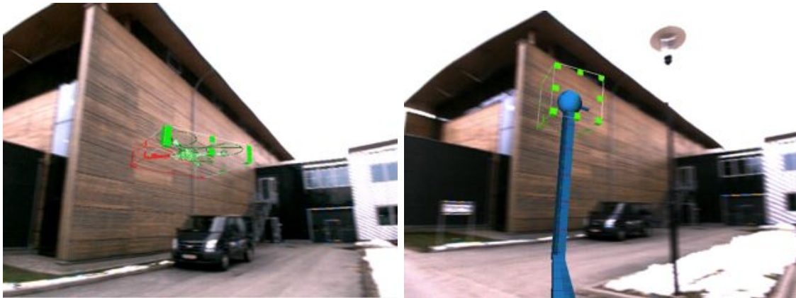
Figure 6.2: Physical vs user-centric virtual cues for MAV navigation. Left) Occlusion cues for a planned waypoint of a MAV. A critical position is highlighted. Right) User-centric virtual cues visualize the distance between the user and the waypoint.
