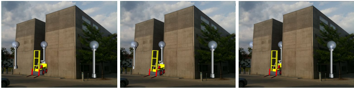
Figure 5.15: Occlusion management using the dense depth map. (Left) Without depth information no occlusion cues can be provided. (Middle) Using sparse geometries for occlusion culling can only create partially correct occlusion and may result in an incoherent visualization. Right) Using dense depth maps for occlusion culling provides important depth cues.
