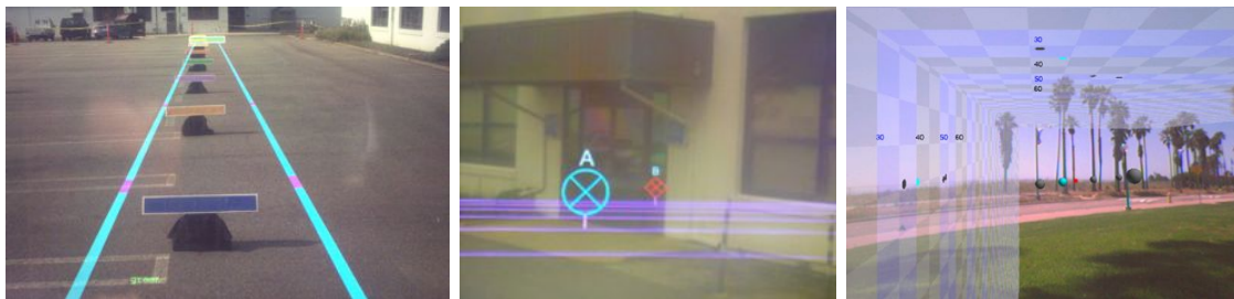
Figure 2.11: Examples for using external virtual cues. Left) Adding a set of parallel lines to improve the depth perception (Courtesy of Livingston et al. [73]). Middle) Using a virtual ground grid to show absolute distances (Courtesy of Livingston et al. [74]). Right) Virtual Shadow Planes for visualizing absolute depths (Courtesy of Wither et al. [118]).
