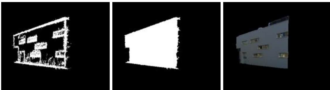
Figure 5.11: Computation of segmentation error. (Left) Reprojected 3D points of the point cloud. (Middle) Computed filled polygon of the reprojected points. (Right) Extracted segmentation.
