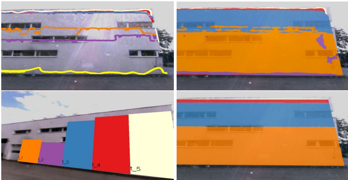
Figure 7.11: Object time overview visualization: providing information of multiple points in time for a single object. The multiple points in time are thereby color coded. Left: Heightlines showing the different height of the wall at different points in time. Middle Left: Geometric Completion shows the completion in geometric reference to the wall. This provides a summary which parts of the wall were added at which time. Middle Right: Completion diagram showing the average completion for multiple points in time. Right: Block diagram showing the average completion of the wall for multiple points in time.
