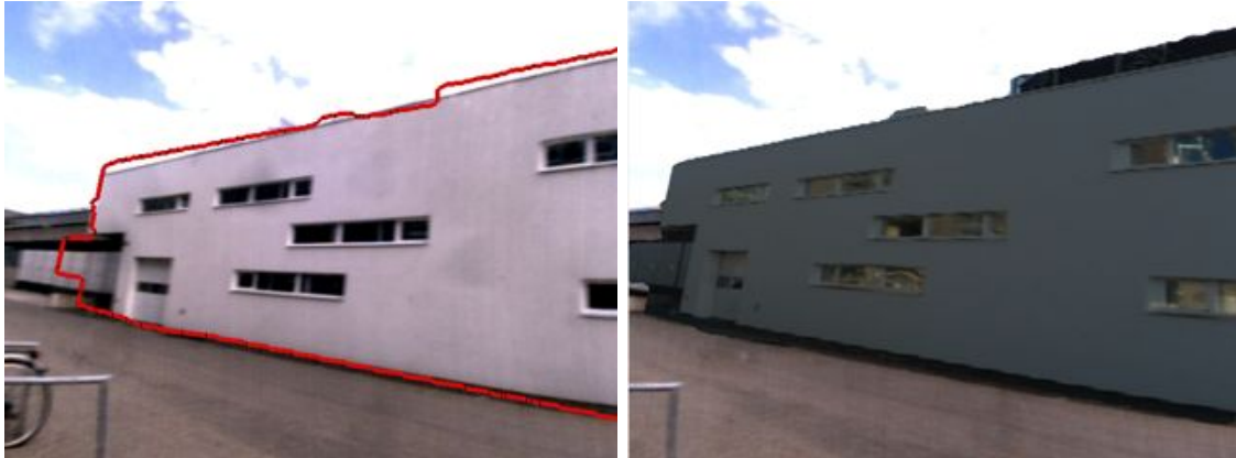
Figure 5.10: Extracted pop-up model in an AR overlay. Left) Outline of a pop-up model overlaid onto an urban scene. Right) Textured pop-up model overlaid on the camera image.
