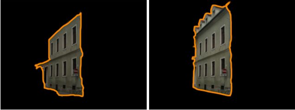
Figure 5.8: Segmentation results. (Left) Segmentation based on the Greedy algorithm, some parts of the roof are missing. (Right) Segmentation based on the Total Variation approach.
