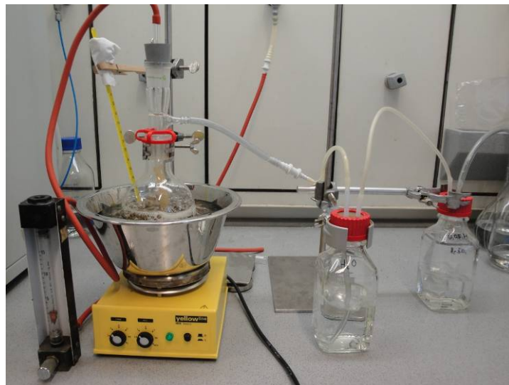
Figure 3-10: Apparatus used for the removal of ammonia from Product 2
