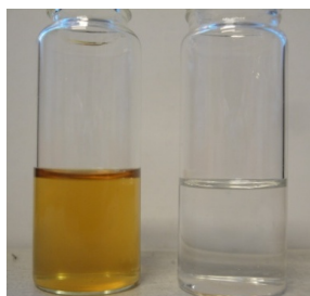
Figure 4-41: Product 1A before (left) and after (right) treating with activated carbon
