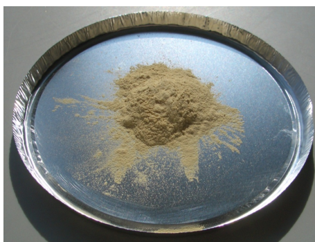
Figure 4-30: AA powder produced by spray-drying
