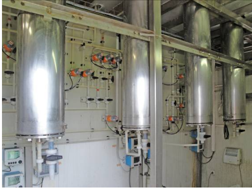
Figure 3-5: IE device at the GBR Upper Austria : column 1-4 made of stainless-steel (left)
