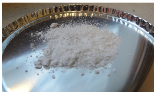
Figure 4-47: Recrystallised BCAA-precipitate from the decoloured Product 1B
