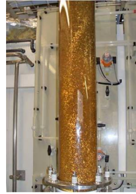
Figure 3-5: IE device at the GBR Upper Austria : column 1-4 made of stainless-steel (left)
