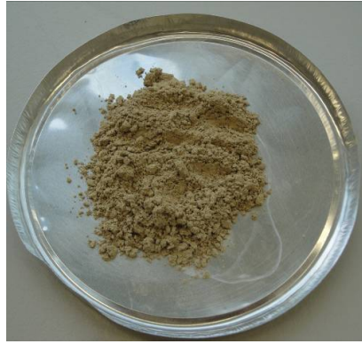
Figure 4-50: AA-powder produced through spray drying of Product 2 from the GRB Upper Austria
