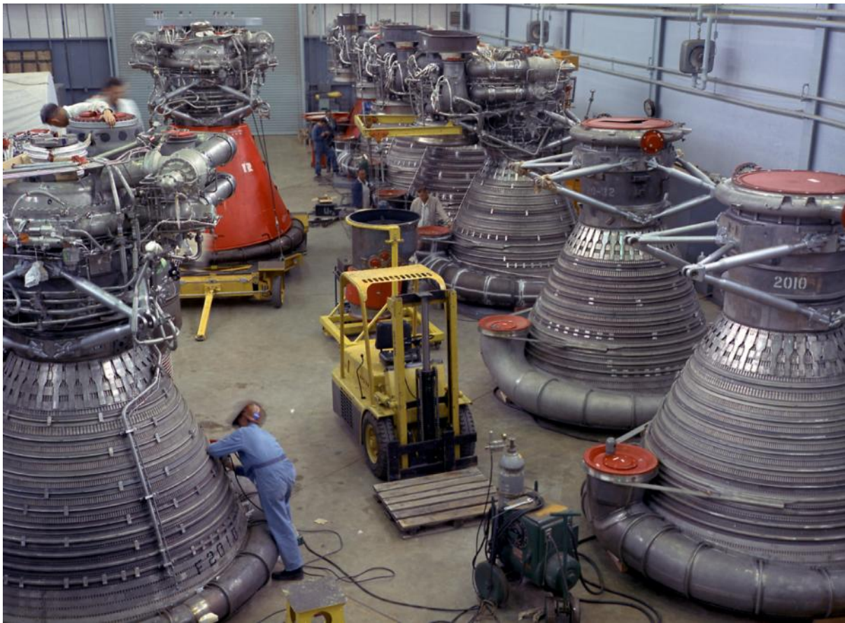
Figure 7-2: F-1 Engines being stored in the F-1 Engine Preparation Shop (Source: NASA)
