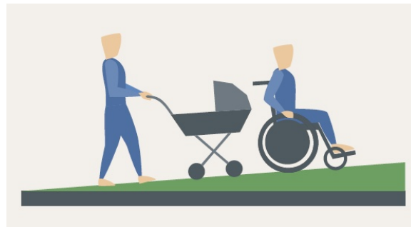
Figure 7.2: Inclination of sidewalk max. 6%
