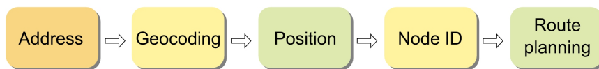
Figure 11.6: Stages from the user input of the address to the start of the route planning algorithm
