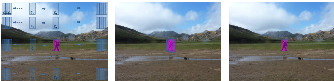
(a) Sliding window technique: one model is tested at each location within the image, often an evaluation with different scales is necessary.
