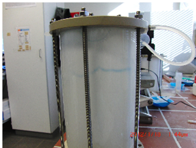
Figure 7.37: Blue dextran ring in annular monolith
