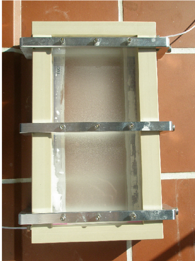
Figure 6.2: Filling frame for the planar test cell with 0.3 mm gap
