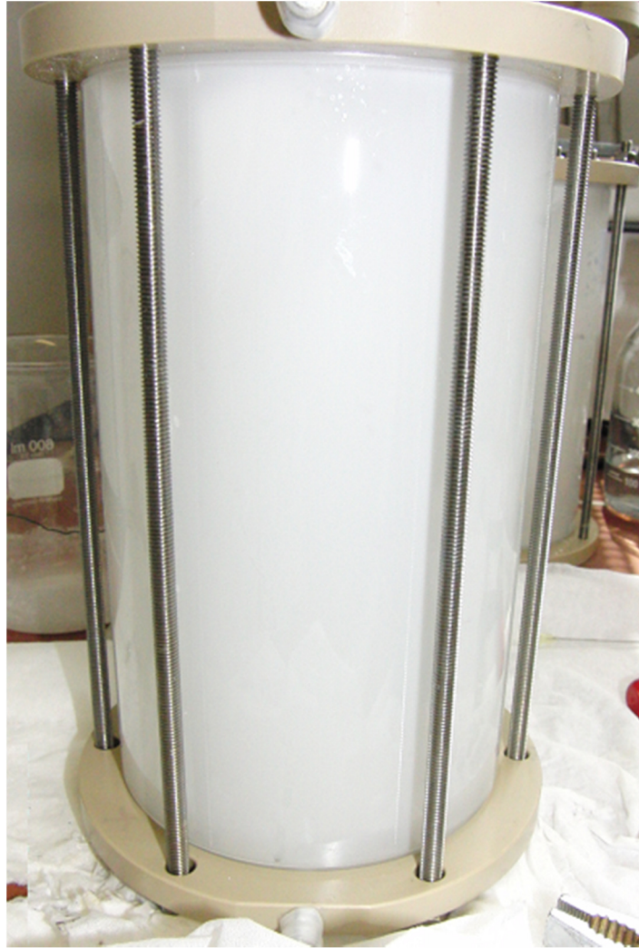
Figure 6.5: Annulus filled with monolithic stationary phase x
