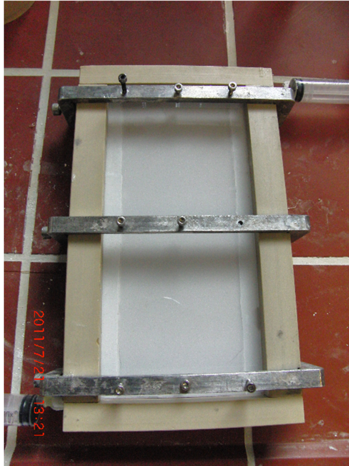
Figure 6.3: Planar test cell filled with monolith in 1 mm gap
