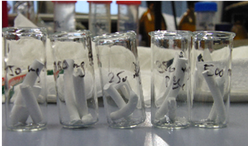
Figure 5.14: Samples for mercury intrusion porosity
