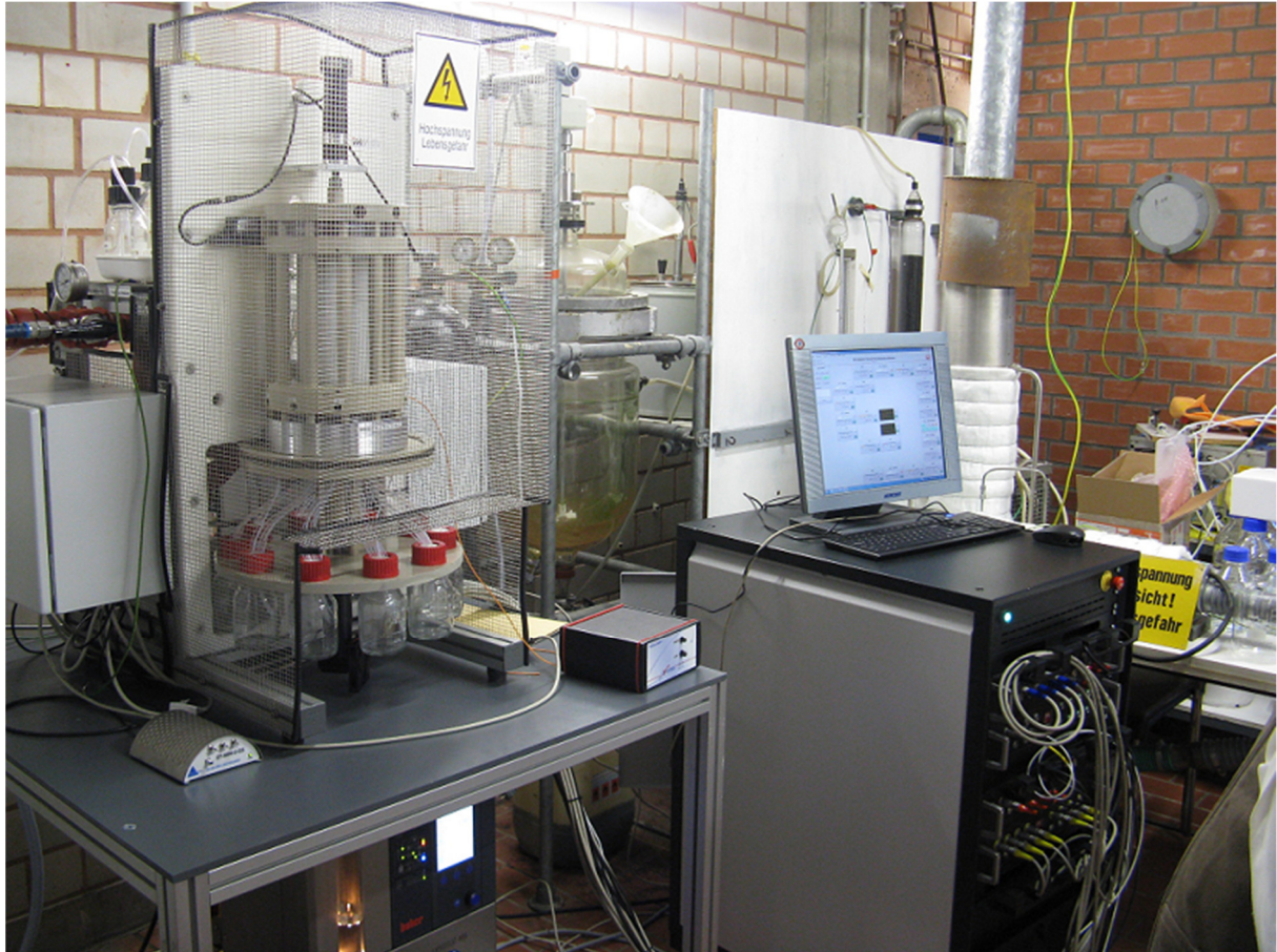
Figure 6.6: Annular prototype with full equipment ready to be operated xi
