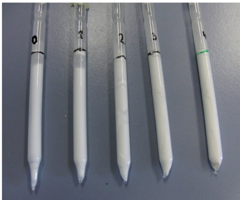
Figure 3.1: Comparison of monolithic precursor mixtures with different weight percentages of silica particles: 0: 0 mg, 1: 5 mg (0.4 w%), 2: 10 mg (0.8 w%), 3: 20 mg (1.6 w%), 4: 30 mg (2.4 w%) silica particles.
