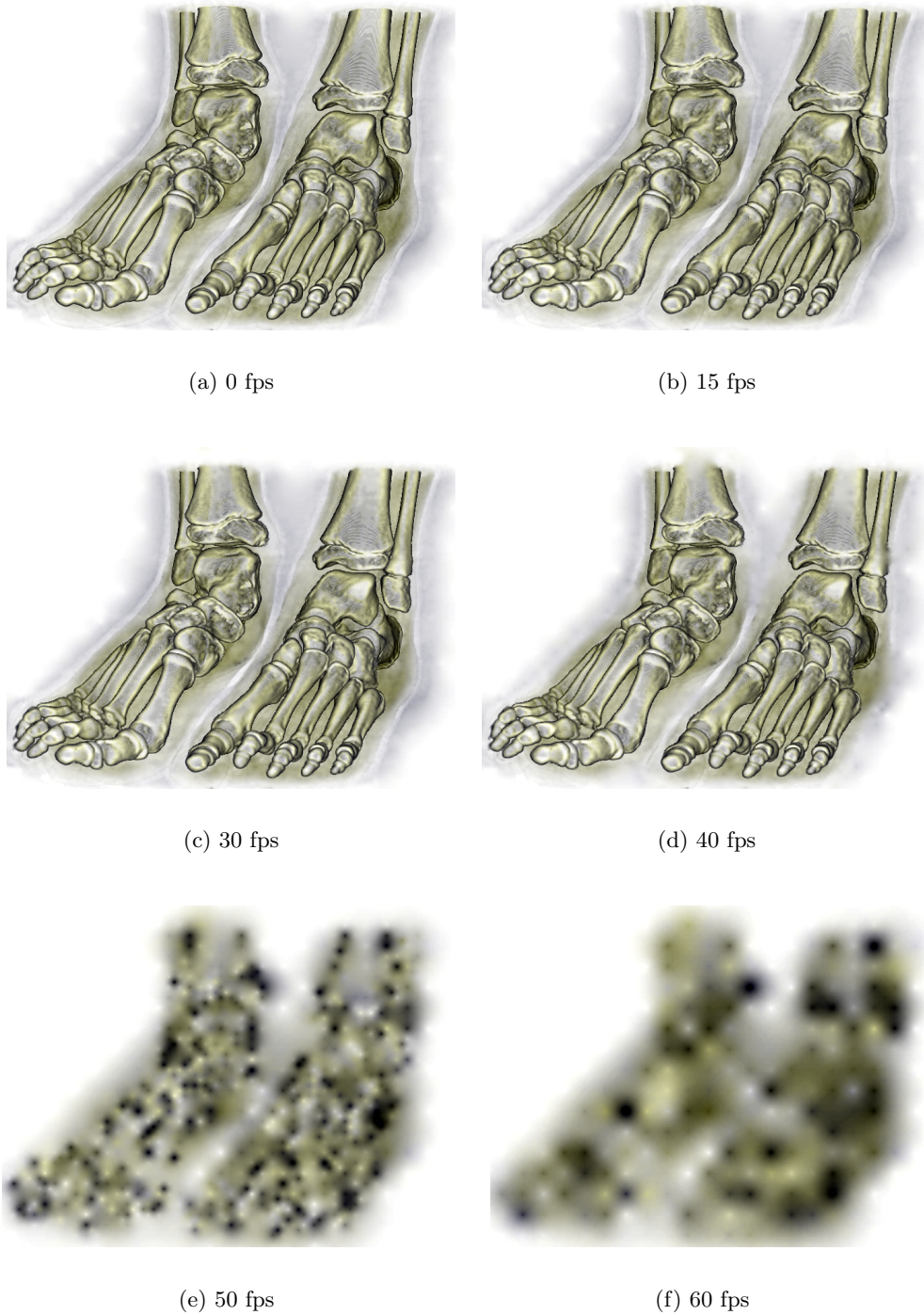
Figure 4.9: This figure illustrates the decreasing quality with increasing requested guaranteed frame rates for a 512^3 volumetric dataset in a 1024 \times 768 viewport.
