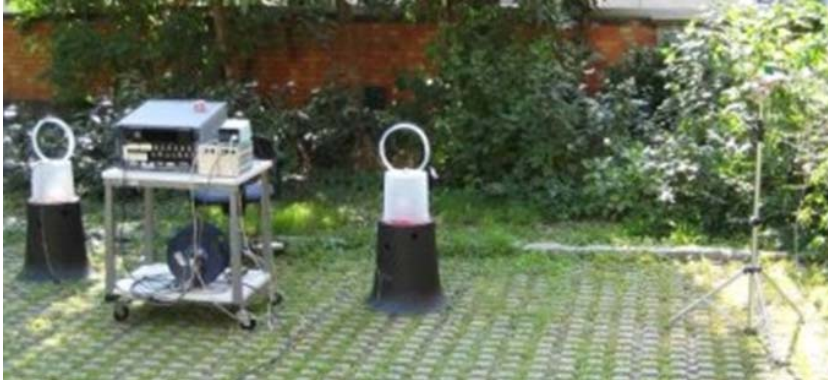
Figure 4.6: Setup by EMT to assess the outdoor eavesdropping distance.
