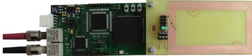
Figure 4.3: A semi passive prototype tag. The 1 st version of the Demotag.
