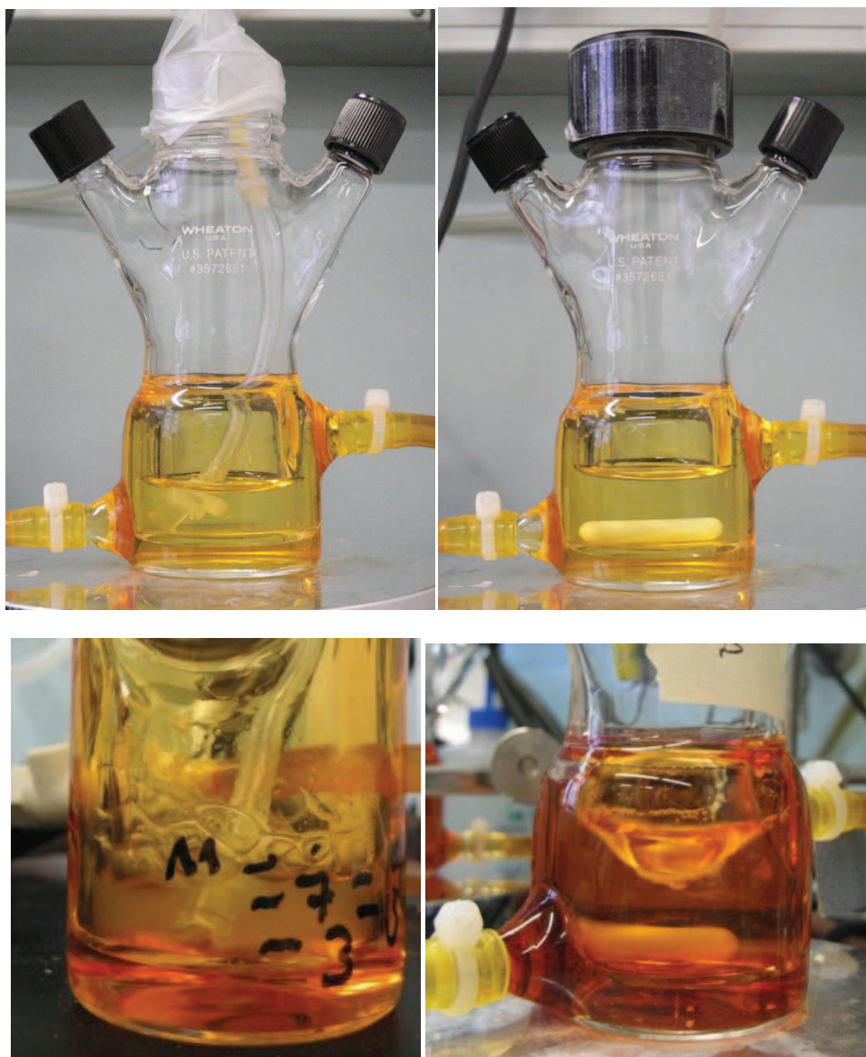
Figure S1: Geometry of the double-walled glass reactors. From left to right: Set-up for bubble aeration and for stirring. Bottom row: Set-up during the accelerated stress conditions bubble aeration and stirring.
