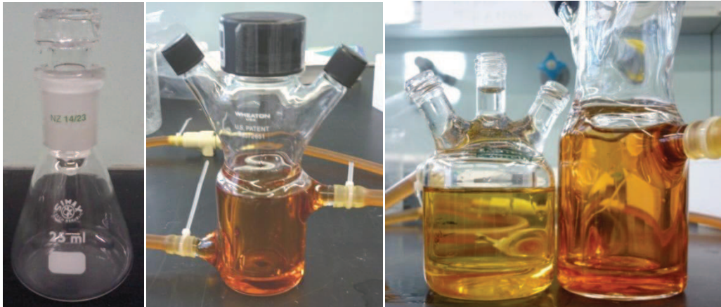
Figure S1: Geometry of the Erlenmeyer flask and the double-walled glass reactors. From left to right: 25 ml Erlenmeyer flask with maximum diameter 4.2 cm and height of 7.0 cm (area 12.0 cm 2 ), double-walled glass miniature bioreactor with a diameter of 3.2 cm (area 8.04 cm 2 ), and comparison with the reactor used for reduced air/liquid interfaces completely filled (area 1.90 cm 2 , three nozzles).
