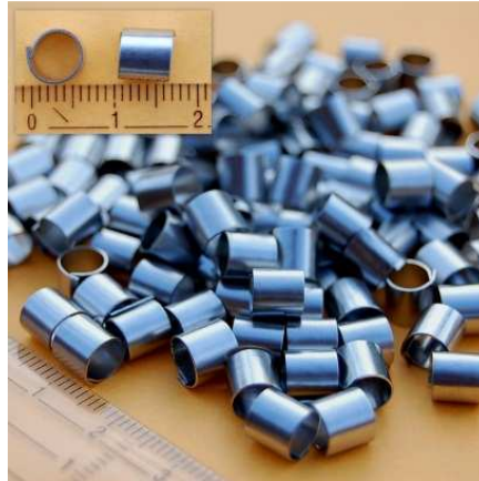
Figure 4-7: Rashig rings of the rectification column
