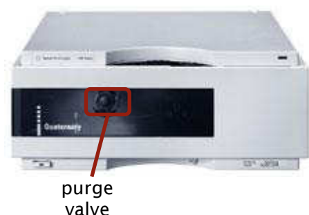
Figure 5: quaternary pump module
