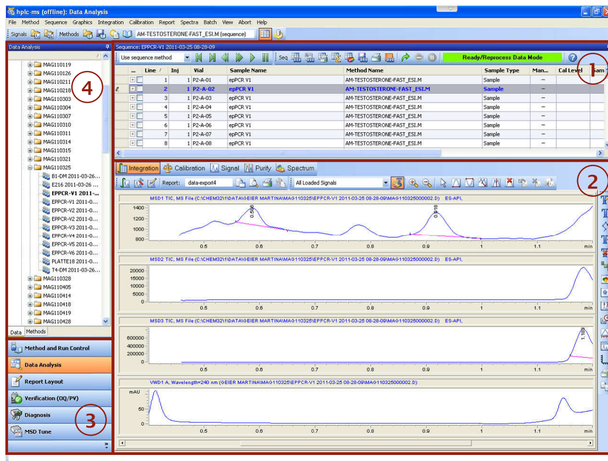
Figure 13: ChemStation: “Data Analysis” screen. sample window (1) signals window (2), task window (3), path window (4)
