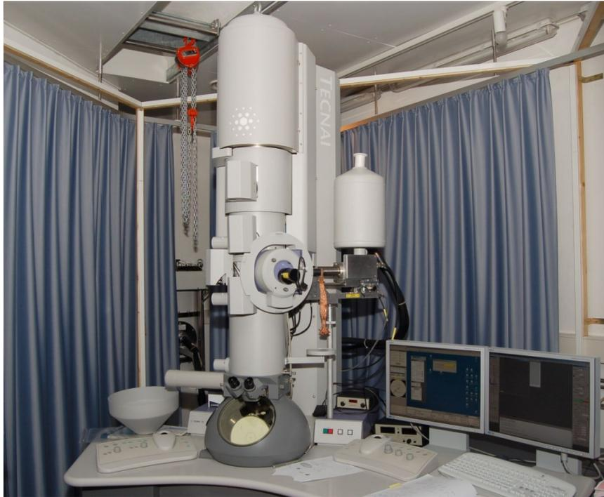
**Figure 2.1:** Tecnai TF20 located at Felmi-ZFE, TU Graz. The TF20 is equipped with a Schottky FEG, Wien type monochromator, EDAX sapphire Si(Li) detector for energy dispersive X-ray measurements, Gatan GIF Quantum with Dual EELS for energy loss measurements, Gatan Ultrascan CCD and Fischione HAADF detector model 3000.
