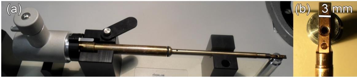
**Figure 4.2:** (a) A Fischione 2040 tomography holder with manual in-plane rotation possibility for multiple axis tomography. (b) A detail of the sample holder. The sample is secured to the holder by the use of flexi-clamps.
