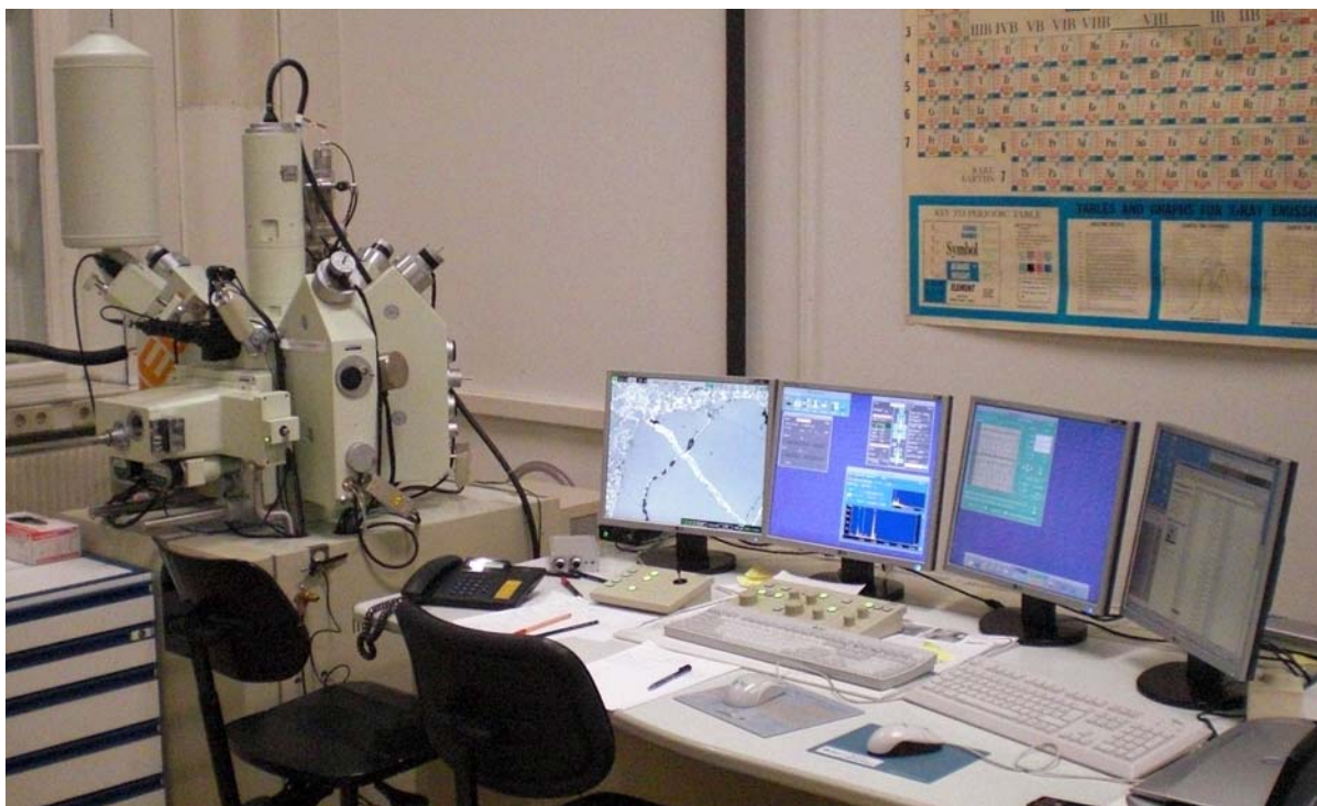
Figure B-2: Microprobe Jeol JXA8200 and work station at the University of Leoben.
