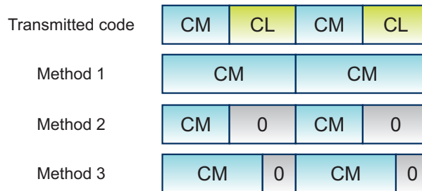
Figure 4.1: Comparison of the different L2C-code generation methods
