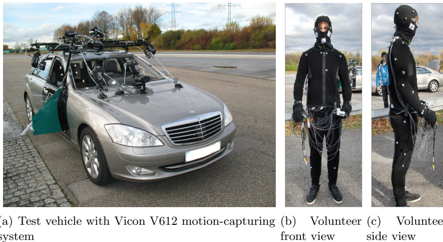
Figure 3.13.: Test series A; vehicle (a) and occupant (b and c), from [HCD + 13]
