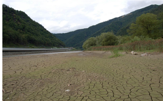
Figure 7.4: View of the cohesive sediment banks in the middle of the reservoir with total lowering of the operation level
