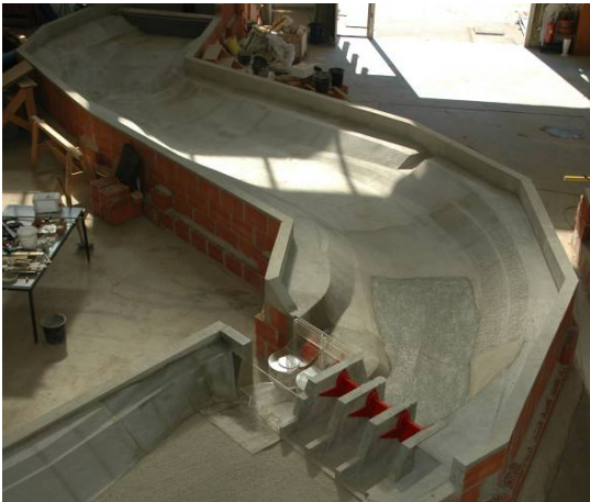
Figure 8.6: A photograph illustration of the physical model with the initial bed level measured in 1973 (Harb et al., 2011)
