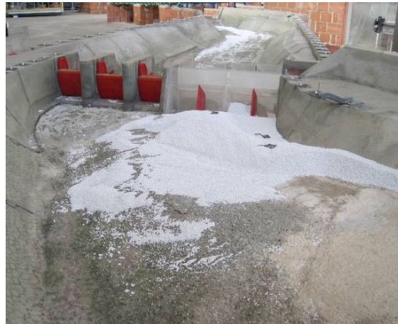
Figure 8.7: Deposited sediment after the test run of a 1-year flood without turbine operation with the measured bed level in 2002 (Harb et al., 2011)
