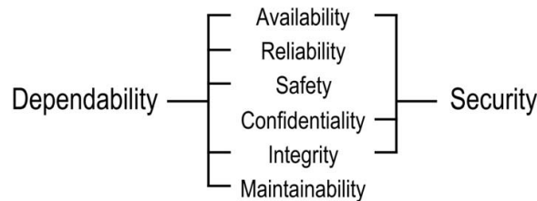
Figure 2.4: The attributes of dependability and security in comparison to each other [ALRL04], highlighting similarities and differences
