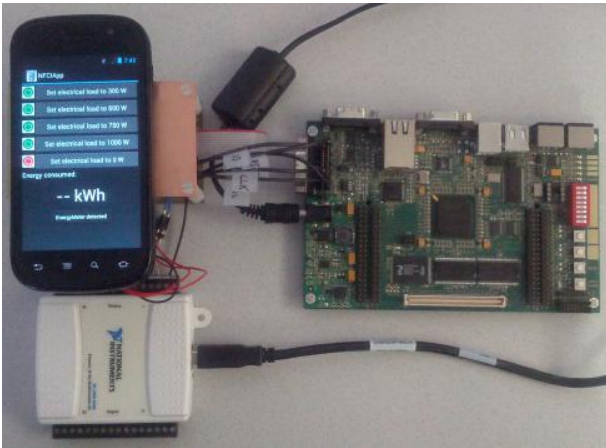
Figure 11. Picture of the prototype built for the case study of using the PtNBridge to interact with a reference implementation of a smart meter.
