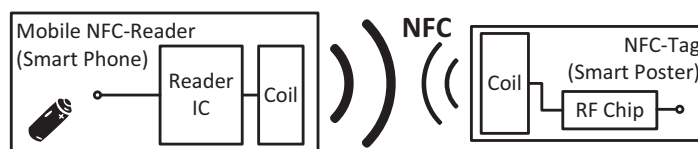
Fig. 8. This figure shows the basic structure of the NFC-System used in the example.
