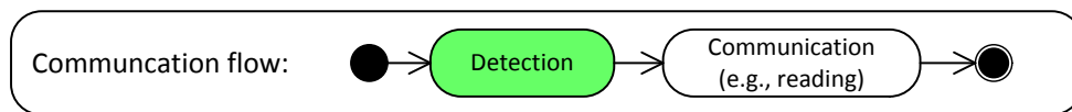
Figure 3.6: Basic communication flow between NFC-Reader and transponder showing in which phase (filled) the magnetic field strength scaling is executed for the first implementation.
