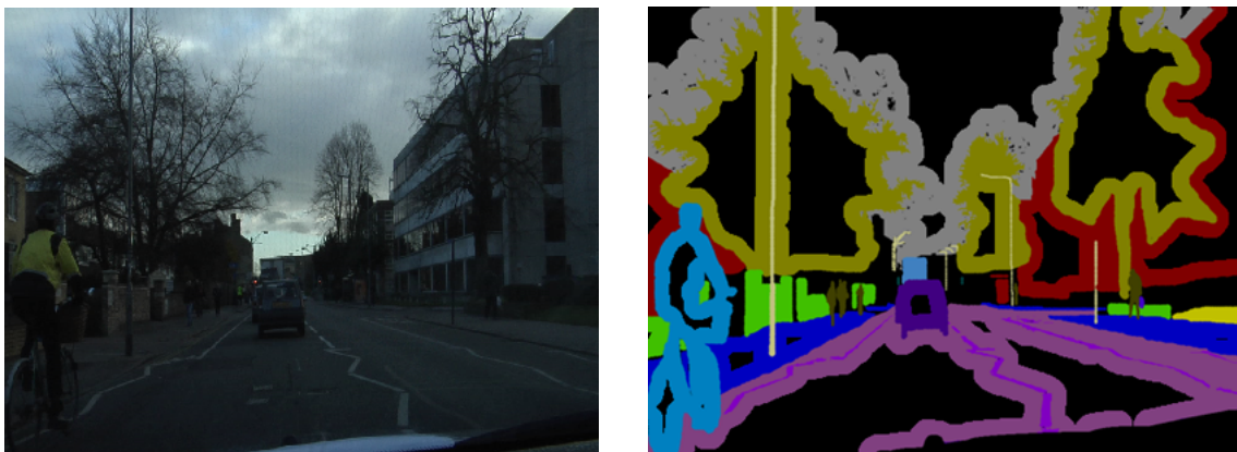
Figure 6.9: Training data examples used for experiments on labelling transitions experiment on the CamVid database. Left: Original image, right: Modified label image showing areas of considered label transitions.
