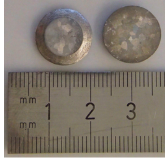
Figure 4.9: Deformed (left) and undeformed (right) Al-3wt%Cu samples after annealing treatment. After etching the grain size in the mm range can be seen by the naked eye.
