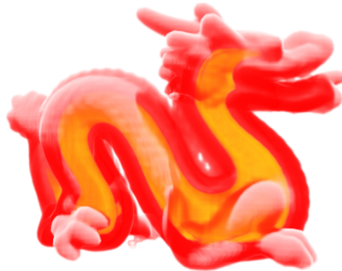
Figure 9.1: The Stanford Dragon, used in the DVR and PBVR case study, is a data set which is simple both in terms of resolution ( 64^3 voxels) as well as internal structure. We use this dataset in conjunction with a simple transfer function for worst-case tests.
