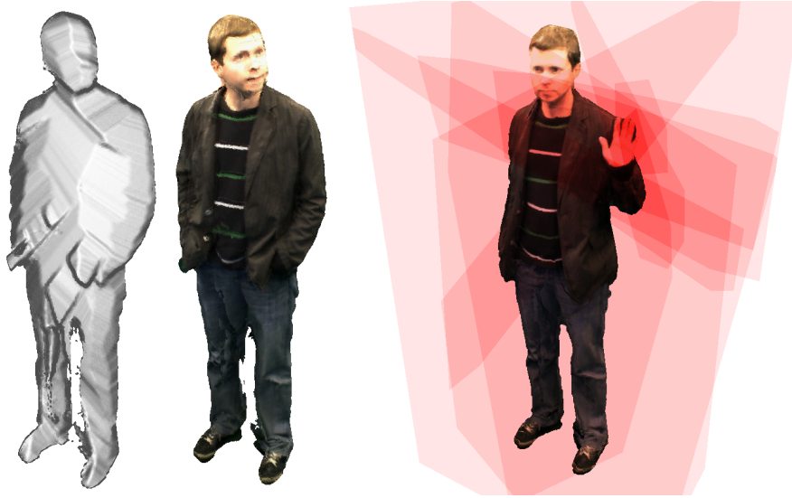
Figure 8.3: A novel viewpoint rendered from 10 camera images by using the image-based visual hull algorithm (left). The redraw buffer encodes the magnitude of change in scene geometry as red intensities, which is directly used as workpackage priority in our Softshell implementation. Images used with permission from Hauswiesner et al. [38].
