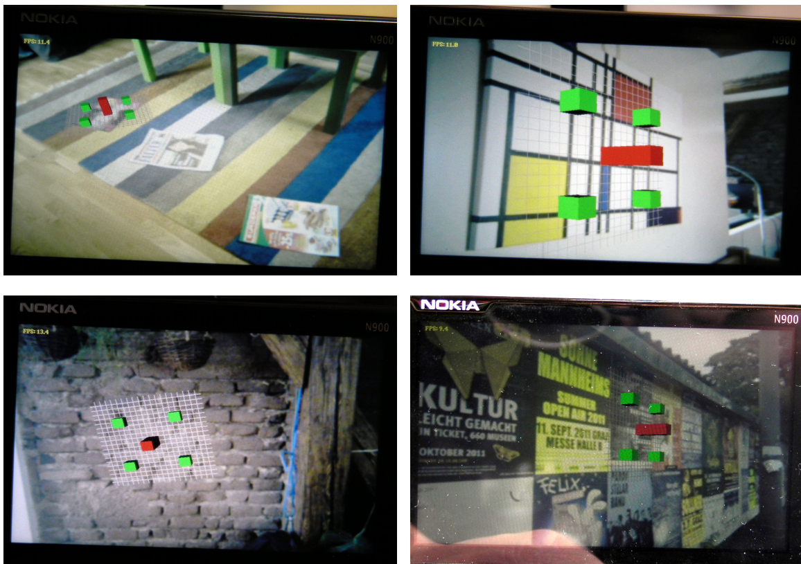
Figure 3.15: Examples of planar indoor and outdoor scenes mapped and tracked with our system (left to right): carpeted floor (with additional texture), wall with tableau, brick wall, outdoor billboard.
