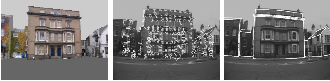
Figure 2.6: The tracking by synthesis method of Reitmayr and Drummond [124] renders a textured 3D CAD model using a pose prior, and performs edge matching with the current frame to estimate an updated 6D pose. © [124]
