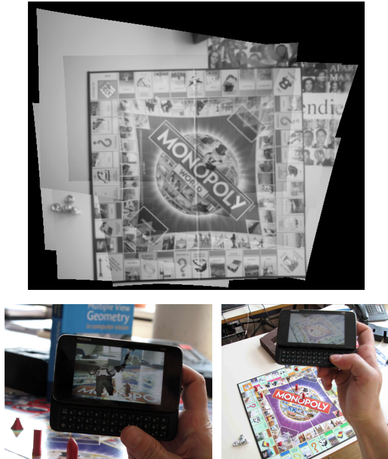
Figure 3.1: Orthoimage sampled from keyframe views of a planar indoor scene and created in real-time on the mobile phone.
