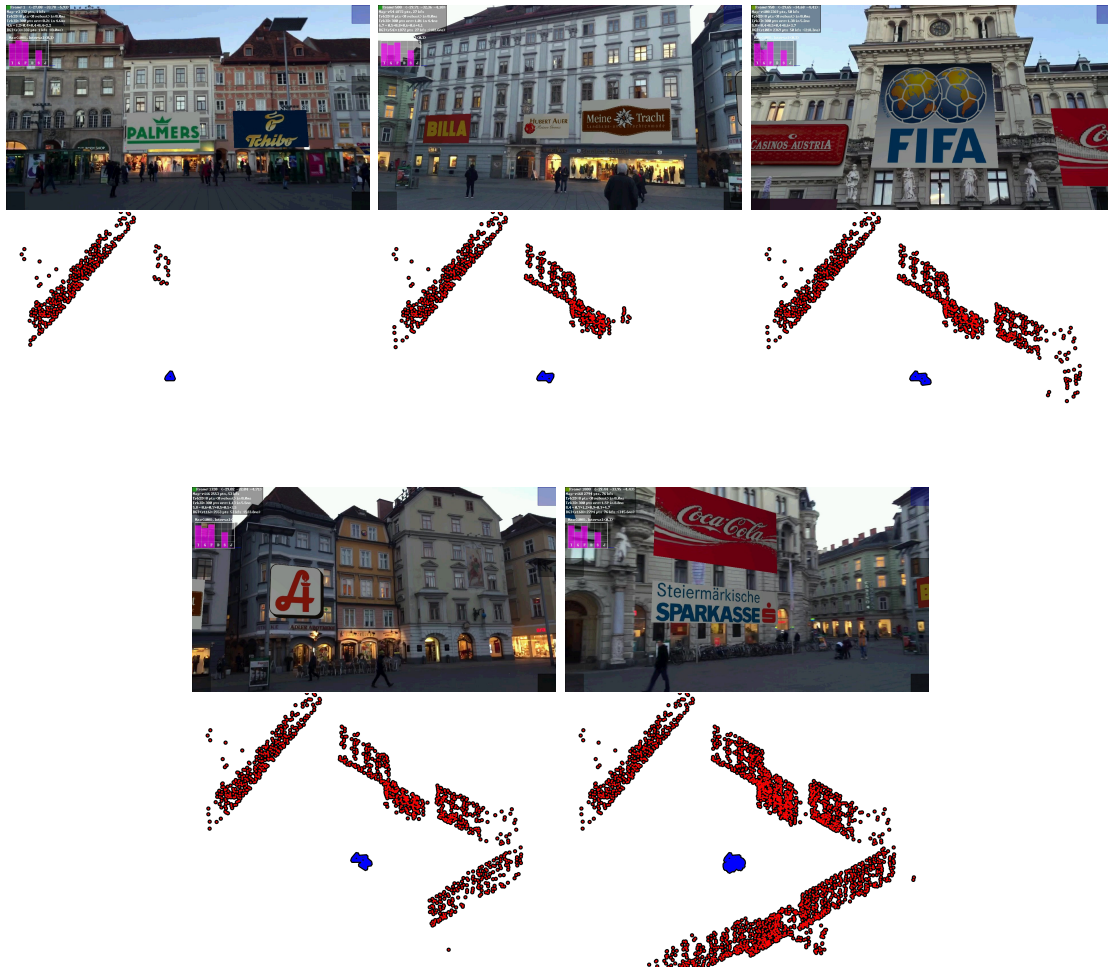
Figure 5.12: Top row: Annotation results from a rotation-only sequence. Bottom row: Expanding SLAM map, while the user rotates a handheld device. The map nicely resembles the structure of the surrounding buildings.
