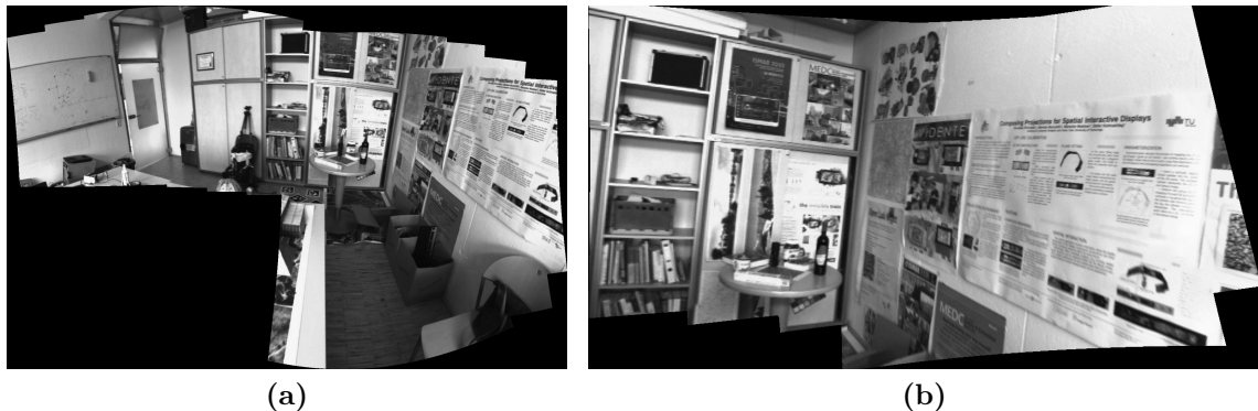
Figure 4.6: Panoramas generated from keyframes of two local panorama maps. The local panorama map (a) was created in the period during frame 800 and 1200. The local panorama map (b) was created in the period during frame 1500 and 1800. Both panoramas depict the scene from two different view points with sufficient parallax for triangulation ( e.g. , the wall on the right-hand side).
