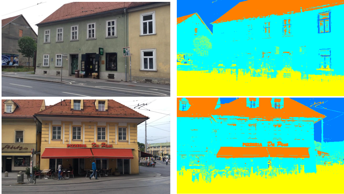
Figure 5.5: Pixel-wise segmentations obtained with a multi-class SVM for two different images. Cyan corresponds to façades, blue to sky, orange to roofs, green to vegetation, and yellow to ground plane.
