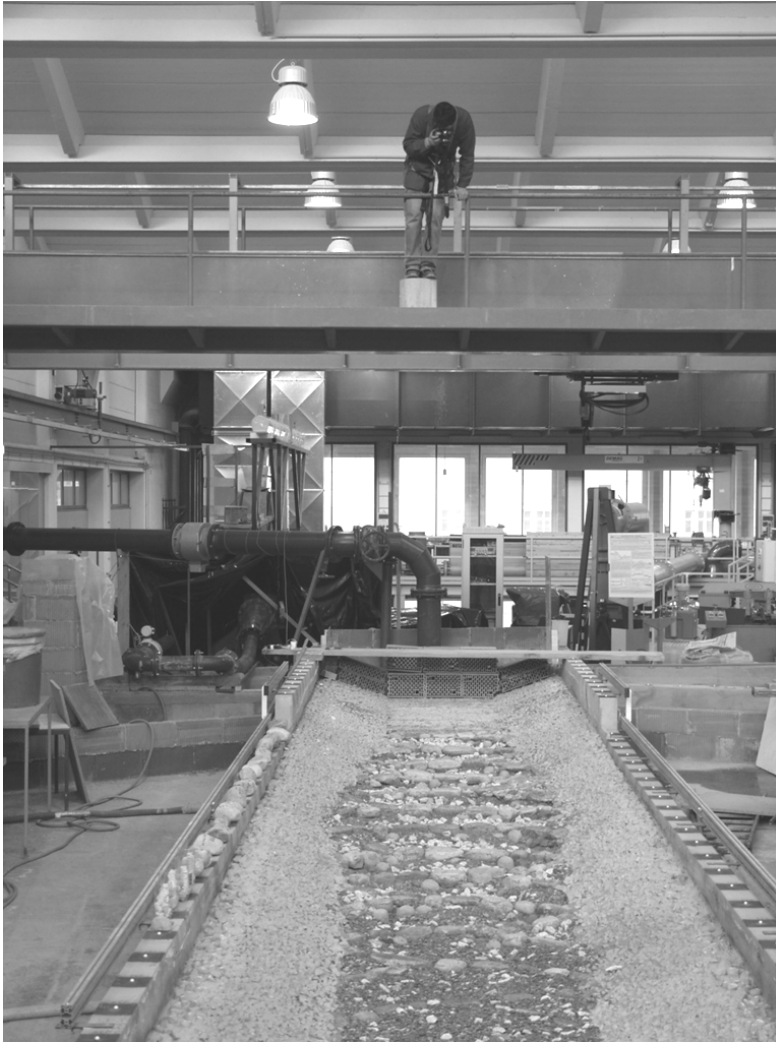
Figure 4.12 Images for digital photogrammetry taken from the crane bridge
