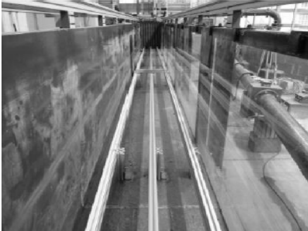
Figure 5.4 Ramp frame constructed from aluminum profiles
