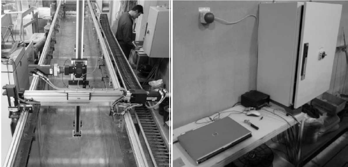
Figure 5.14 positioning system (left), measurement cabinet with control unit (right)
