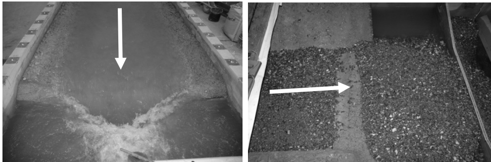
Figure 4.42 No flap, overfall into the sand trap (left) wooden board at the downstream end of the sand trap (right)
