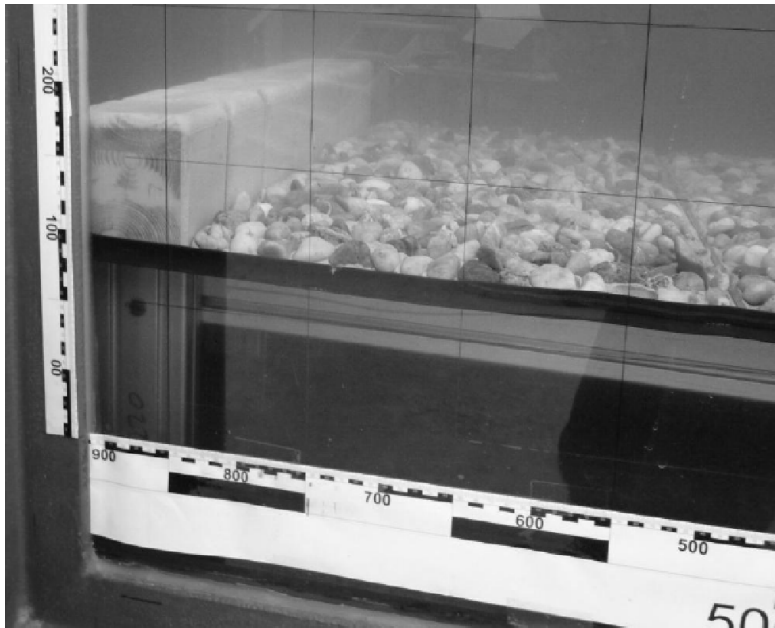
Figure 5.5 Elements comprising the ramp construction (side view): longitudinal profile, vertical column, roughness elements, panels with gravel, rubber seal
