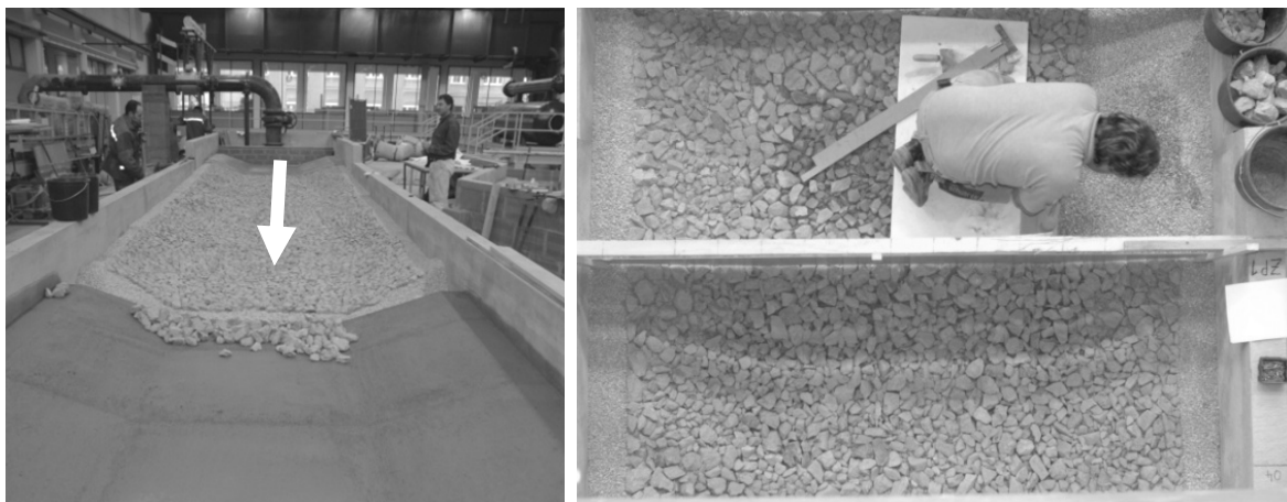
Figure 4.15 Construction of the model: view from the downstream end of the model (left), pavement of the bed with coarse gravel (right)
