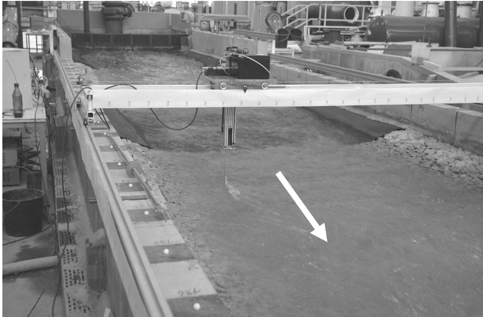
Figure 4.9 Carriage for ADV-probe moving on rails
