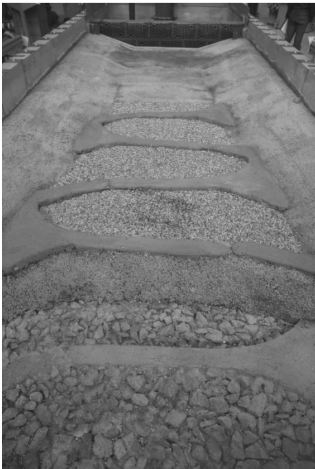
Figure 4.19 Ramp design D2
