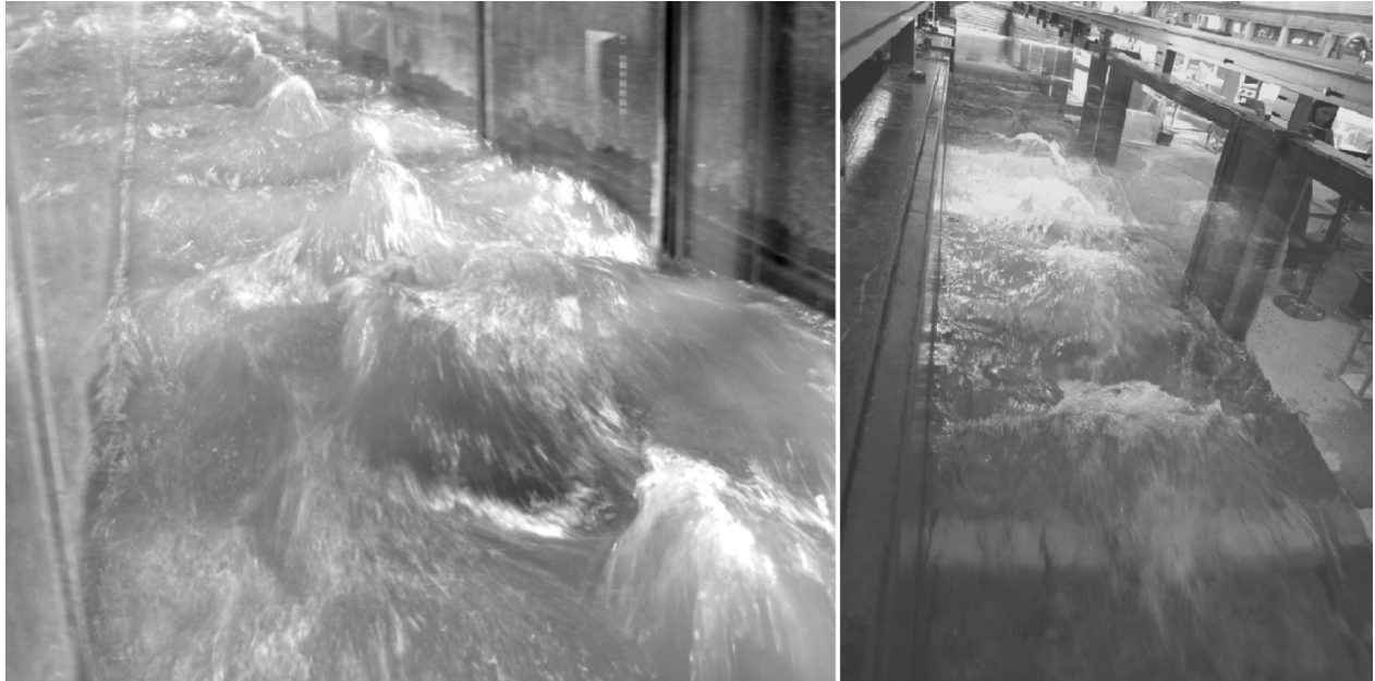
Figure 5.59 Flow Pattern 3D-Antidunes (Núñez-González, Martín-Vide 2010) (left), Rapid Flow for variant: I25-K8-L80, rough bed, flow from background to foreground for both pictures
