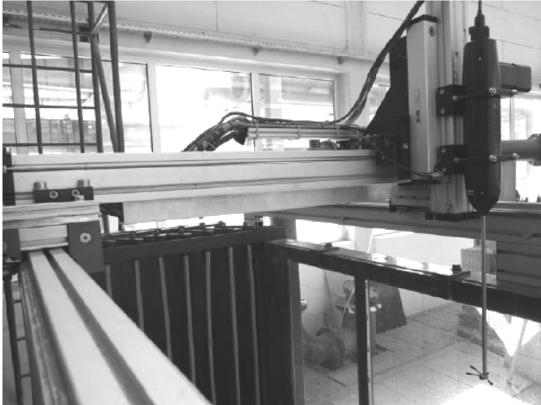
Figure 5.12 Side-looking ADV-probe “Vectrino” on positioning system at the downstream end of the flume
