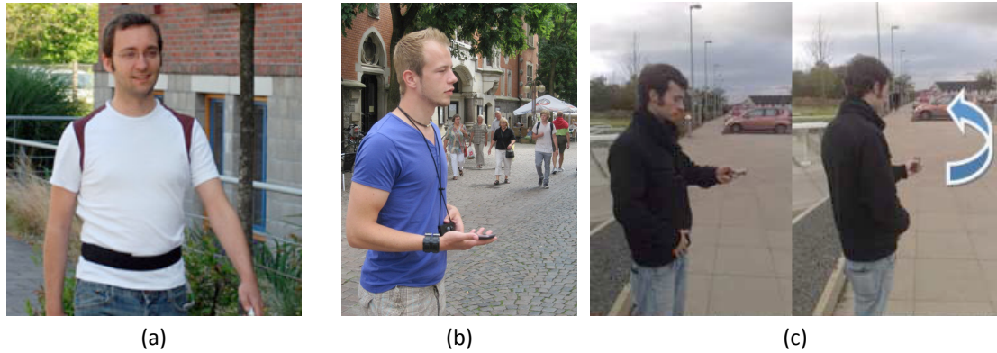
Figure 2.6: Multimodal interaction with handheld navigation systems. (a) Adding a vibro-tactile belt to communicate the direction of waypoints in the environment (Pielot et al. [141]). (b-c) Pointing as an input metaphor to explore the information in the surroundings (Pielot et al. [142], Lei et al. [93]).
