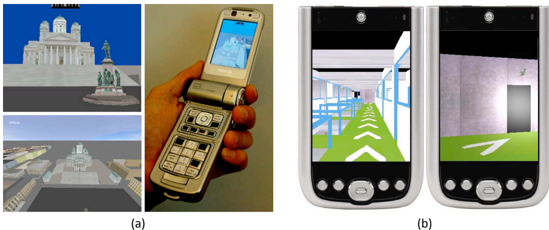
Figure 2.5: Use of 3D maps in handheld navigation systems. (a) Oulasvirta et al. [133] study the use of 3D maps in outdoor settings, discussing differences in usage between street-level views and bird's eye views. (b) Chittaro et al. [25] explore the use of 3D maps indoors, as a support for building evacuation.
