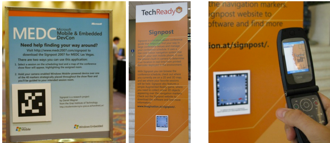
Figure 8.2: Marker-based localisation with Signpost. Left: posters and fiducial markers deployed at the MEDC 2007 and TechReady7 conferences. Right: our localisation system at TechReady7: a user points the phone towards one marker, until the marker is recognised and the system updates the map highlighting the user's position.
