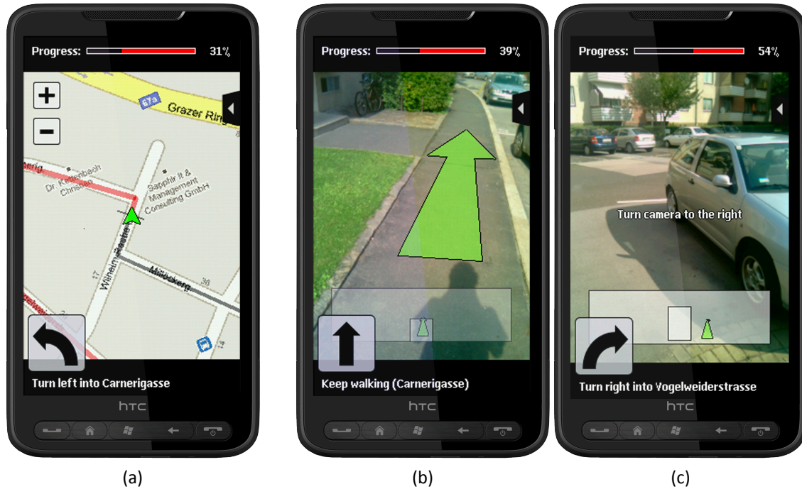
Figure 7.1: Screenshots of our prototype. (a) We employ maps, glyphs and text instructions to provide information about the path and the next turn. (b) We augment the physical world with arrows to provide egocentric navigational cues. (c) When the augmentation is not visible, visual cues guide the user in pointing the camera to the right direction.
