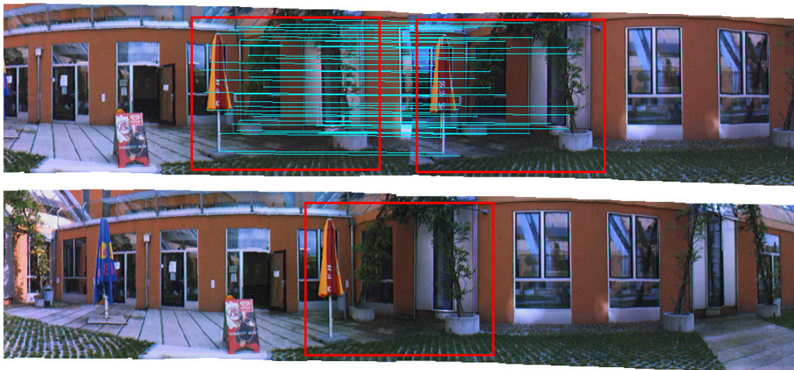
Figure 4.3: The typical output of our panorama tracker before and after loop closing. Top: a full 360° loop with overlapping areas highlighted. Bottom: the same panorama after the application of our loop-closing procedure.
