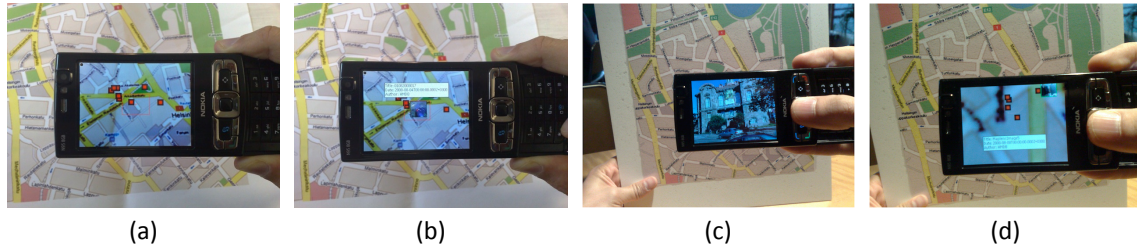
Figure 6.1: The first prototype of MapLens. Typical interaction with the information: (a) browsing images on the map, (b) hovering the phone over an icon shows a thumbnail of the corresponding image, (c) clicking on a thumbnail shows a full-screen version of the image, (d) when icons are cluttered, users can freeze the video view and magnify it.
