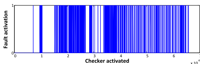
Fig. 4. Checker result trace - CPU startup and AES encryption
