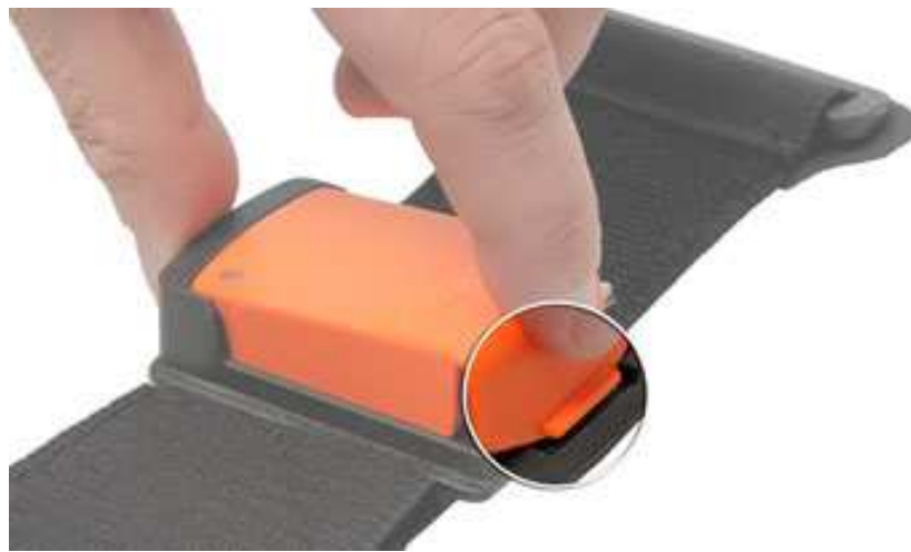
Figure 6: portable IMU MTw development kit (xsens)
