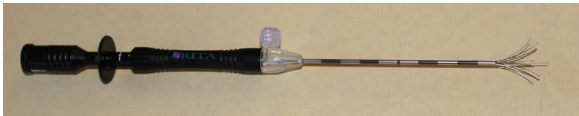
Figure 7.3: The RITA Starburst device: in this picture the array is deployed to an extension of 3 cm as used for the animal study. So this is the structure visible as the needle in the animal CT scans.
