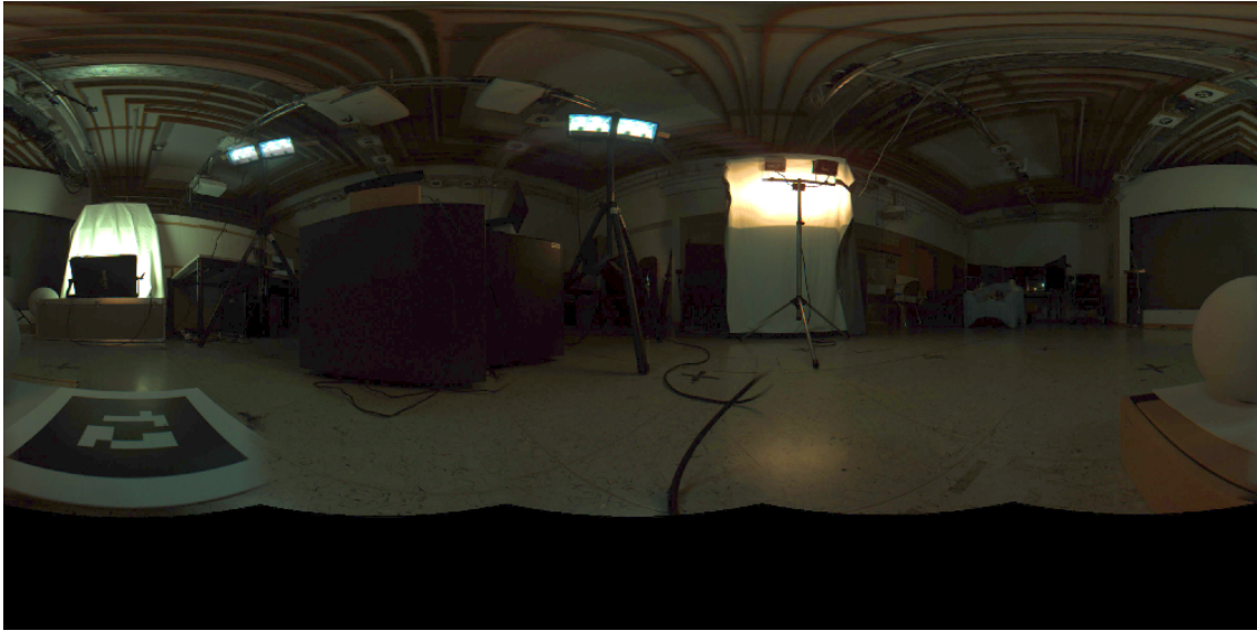
Figure 3.4: This figure shows a panorama image of the controlled lighting environment. There are two directed light sources in the middle and two indirect light sources on the left and on the right of the panorama. This image has been created by an omnidirectional camera (Ladybug3).
