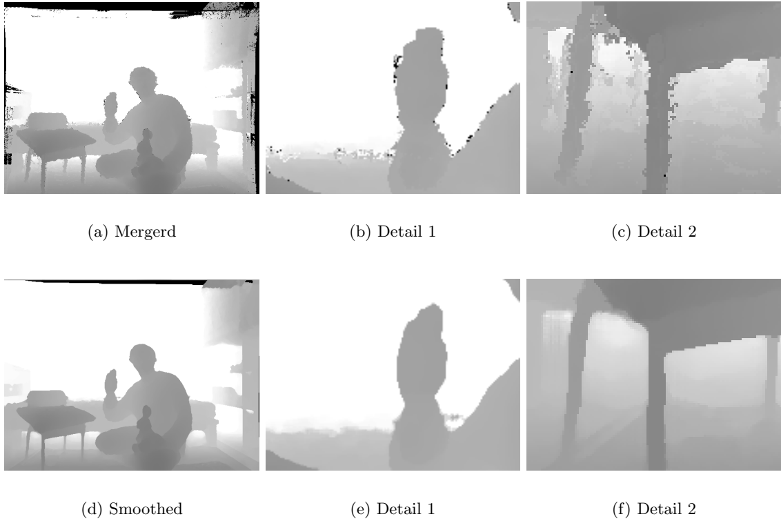
Figure 4.6: The middle and bottom columns show close-up views of the first column. Note the significant improvements in depth edges along the borders of objects, such as the chair legs, after applying our filter pipeline.
