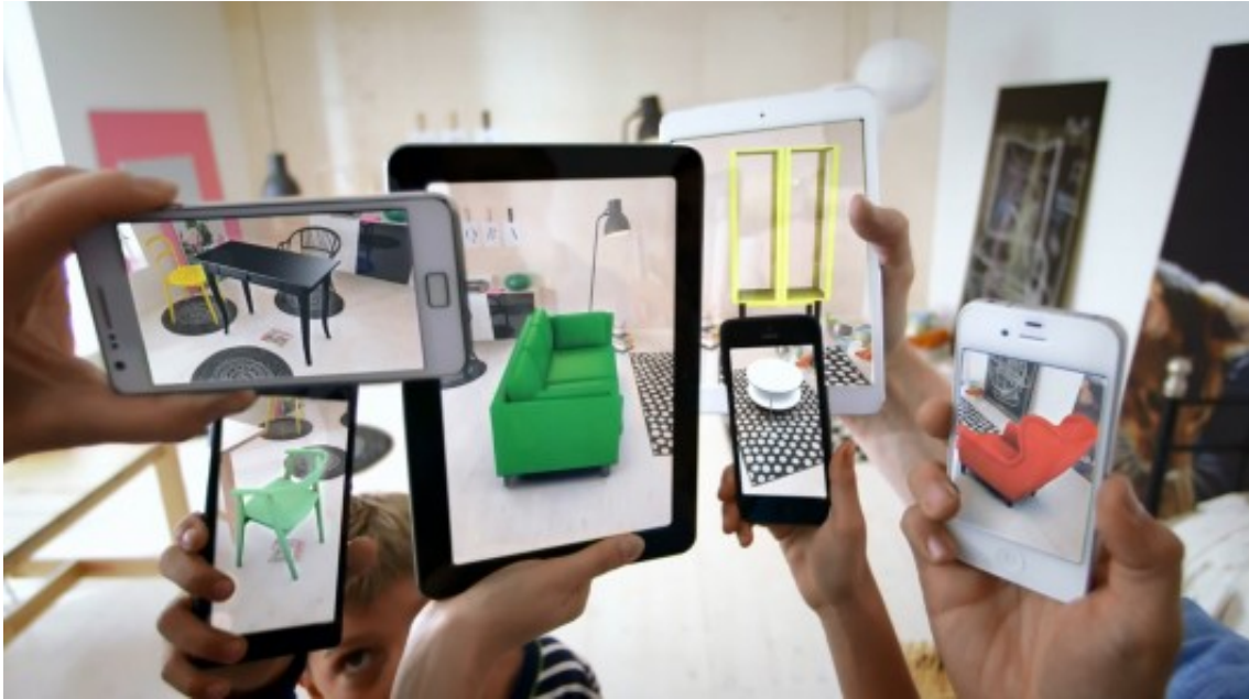
Figure 1.1: Example of an Augmented Reality "home shopping" scenario created by IKEA. Users perceive the real-world captured by a camera through the display of their mobile devices. Over the camera image virtual furniture is rendered. Due to camera tracking technology the virtual object stays in place even if the devices move, creating the illusion of being attached to the real-world. Photometric registration is not handled in this solution. If the lighting condition of the room would change, the appearance of virtual objects would stay the same.
