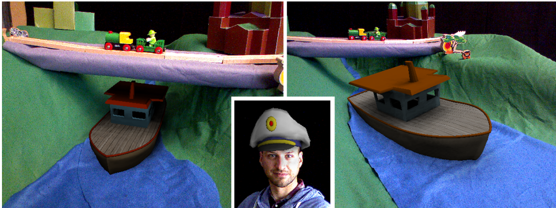
Figure 8.2: Left image: real-world bridge casts a shadow onto the virtual ship and the virtual ship casts shadows onto the real-world environment. Right image: the direction of the virtual shadows can be compared with the real-world shadows, as cast by the little lion, for example. Middle insert: we added a virtual hat onto the head of a real person to demonstrate the ability of the system to work in unprepared environments, too.
