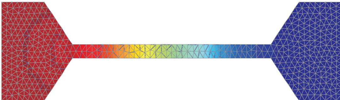
Figure 5.2: Electrical potential distribution
