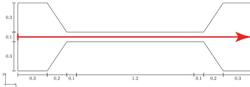
Figure 5.10: Cross-section through feeders and heating plate for evaluation of the results
