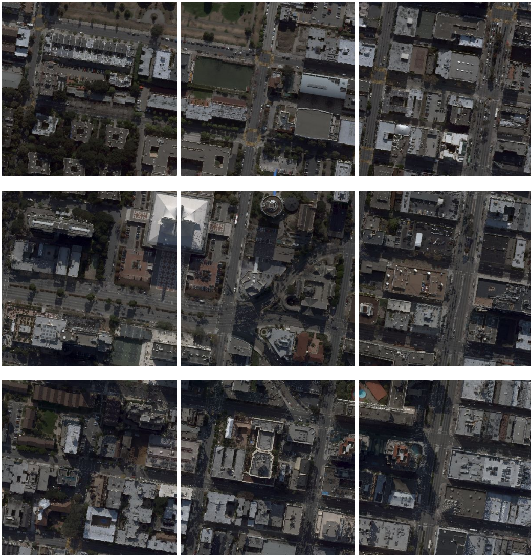
Figure 4.19: Some wavelet-based fusion result computed for a small part of San Francisco , where every pixel describes a point on ground with a size of 15 cm.
