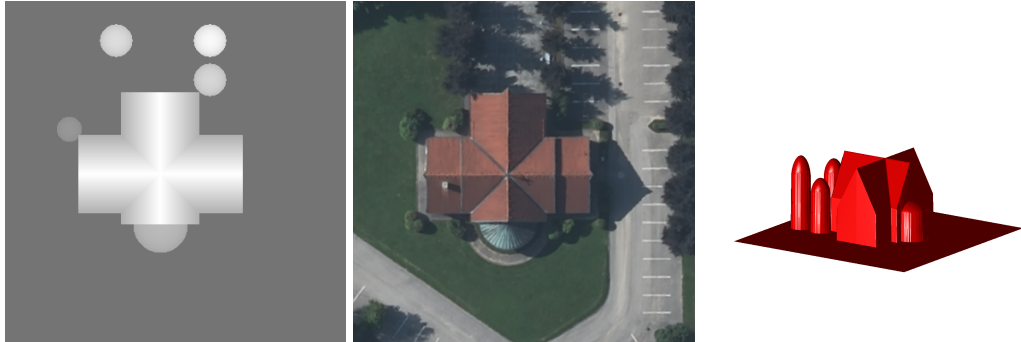
Figure 4.7: A synthetically generated height model to evaluate the performance of our fusion model. From left to right: the height model, texture information and a rendering of the synthetic setup. We add artificial noise to the height field in order to produce multiple input observations. Since the ground truth is provided by the original model a quantitative evaluation can be performed in terms of the PSNR. We use a small amount of Gaussian noise, impulse noise and varying percentages of undefined pixel information.
