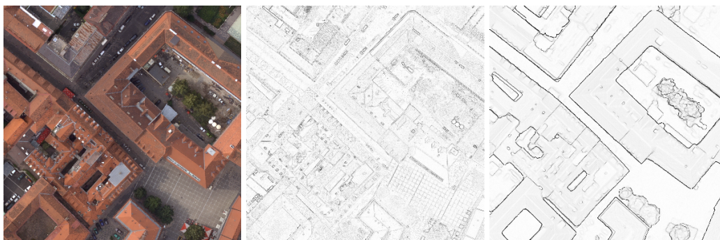
Figure 4.6: A computed penalty function for an arbitrary aerial scene. We derive the edge image either from color or height data. In particular for elevated objects the penalty terms, computed from height, will give an improved object delineation, since shadows and color changes may produce irrelevant edges.
