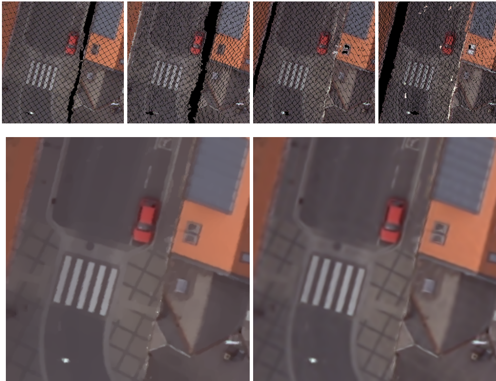
Figure 4.15: Obtained fusion results for a detail of Graz . The first row shows redundant scene observations with many undefined pixels, mainly caused by occlusions and sampling effect. Both the TV-L^1 (left, second row) and the wavelet-based fusion model (right, second row) obtain accurate results, however the image-priors provided by the wavelet decomposition shows an improved appearance.
