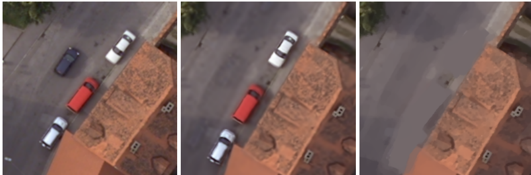
Figure 4.20: Car inpainting by using constant color priors. From left to right: The original perspective image, the fusion result without using a car detection mask and the inpainting result obtained and for the wavelet-based model.
