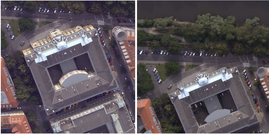
Figure 2.8: An orthographic representation for a Graz scene. While the left image shows a perspective view, the right one depicts the ortho-photo of the same scene, where the parallel projection yields constant pixel sizes. It is obvious that vertical structures, like facades, disappear in the ortho-view.
