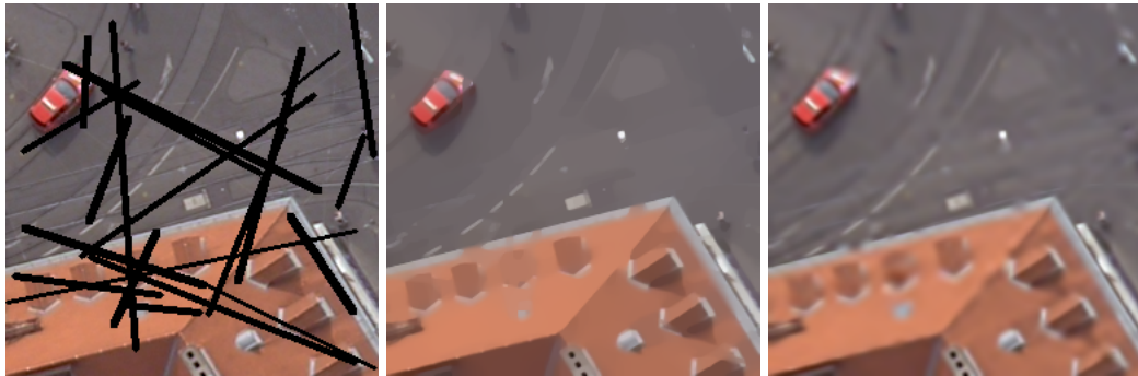
Figure 4.12: Image recovery from a single input observation, which is distorted with random lines. From left to right: the noisy image, the inpainting result computed with the TV- L^1 model and the result obtained with the wavelet-based model.
