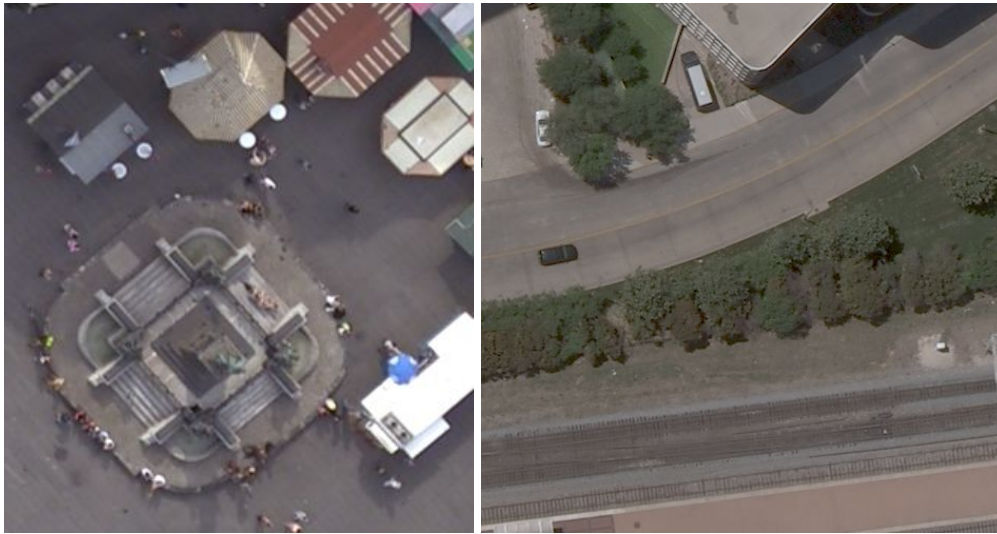
Figure 1.1: Small image patches cropped from huge digital aerial images at pixel sizes of 8 cm and 15 cm, respectively. One can notice that fine image details, such as walking people, vegetation or railway tracks are preserved accurately.
