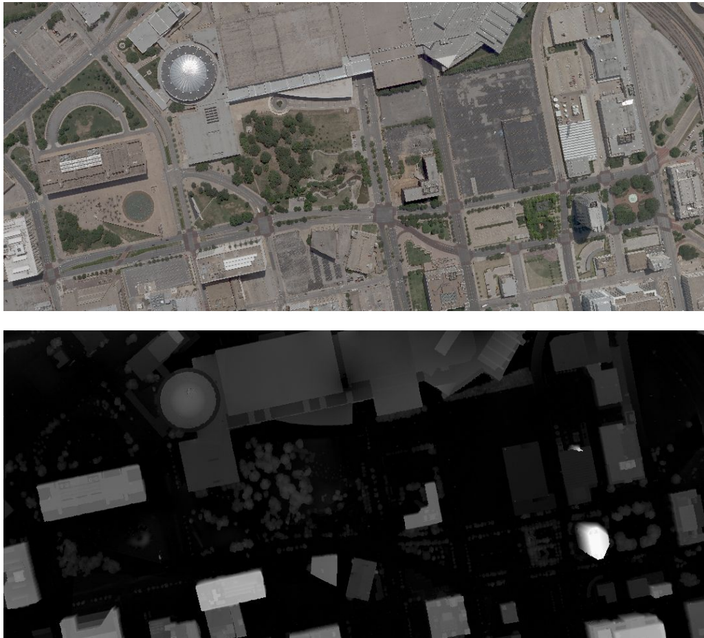
Figure 2.7: Elevation measurements for an image of Dallas . The computed elevation maps provide absolute height values for each pixel. Dark values denote no elevation, while bright color defines high elevation. Such normalized surface model are widely adopted for 3D modeling, however, in this work we extensively utilize this representation for the generation of a full semantic interpretation.
