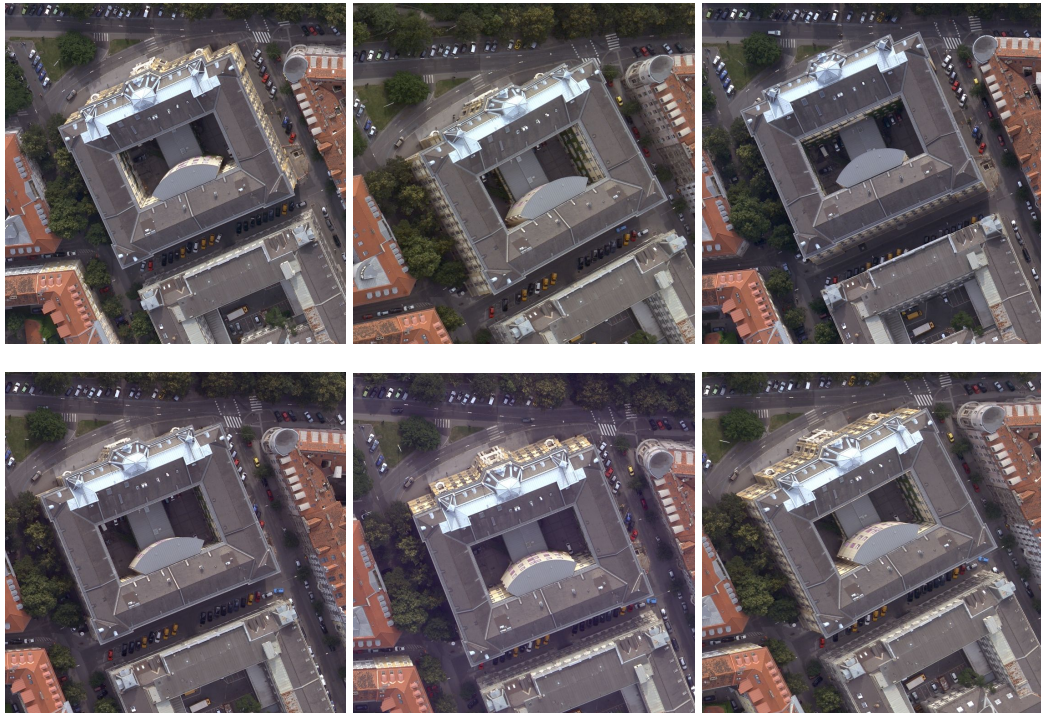
Figure 2.3: Some redundant observations of a scene located in Graz . The mapped area is shown from different camera viewpoints, which are defined by the flight direction. In our approach we integrate overlapping information within a common orthographic view.
