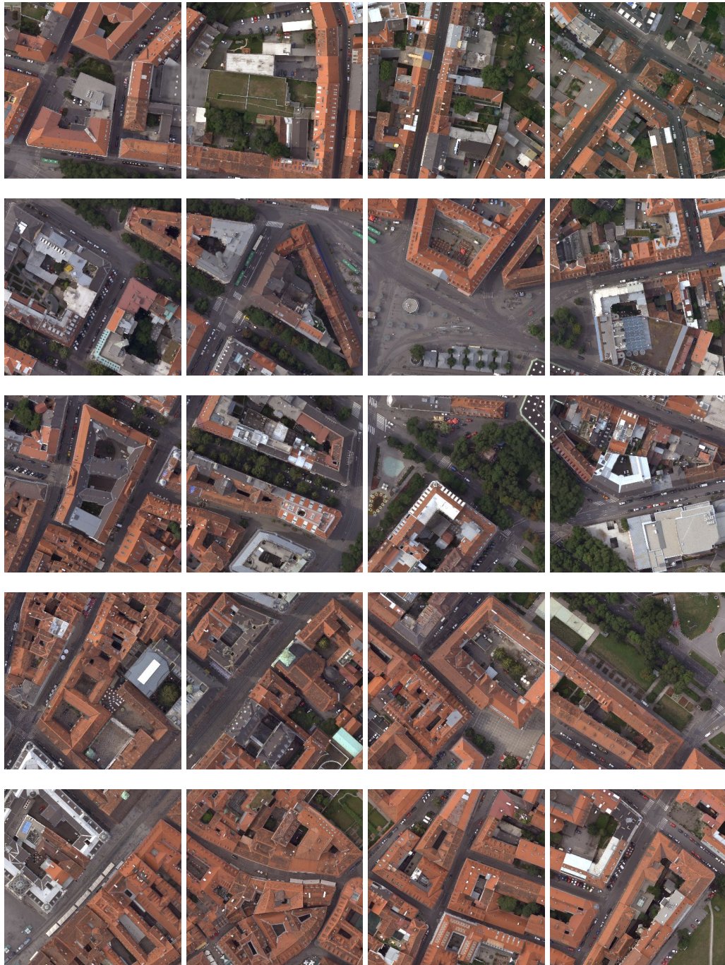
Figure 4.18: Some wavelet-based fusion results obtained for the inner city of Graz . We compute the fusion for image patches with a size of 1600 \times 1600 pixels. Every pixel in the image patches represents a point on ground with a size of approximately 8 \times 8 cm.
