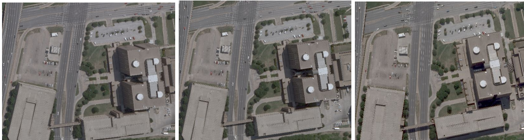
Figure 3.1: Highly overlapping aerial images taken from Dallas . The mainly gray-valued areas provide a challenging task to discriminate, e.g. , building structures from the street network. We thus argue that 3D information has to be integrated for an accurate semantic scene interpretation.
