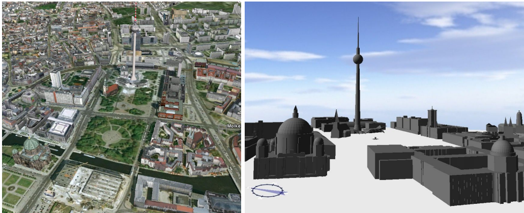
Figure 1.2: A scene of Berlin rendered and visualized in Google Earth (left) and the corresponding CityGML model (right) with overlaid buildings, represented in LoD 1 to 3. Note that both models have been generated with massive human interaction.
