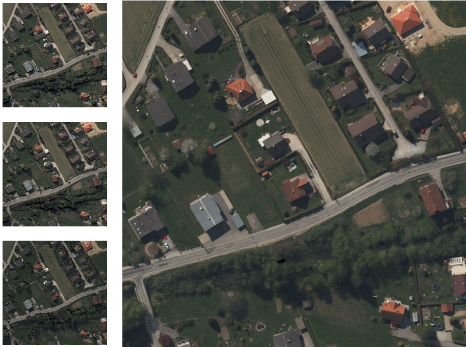
Figure 4.17: A wavelet-based fusion result for a larger region ( 128 \times 128 meters). We integrated a total number of 8 redundant scene observation. Note that the fusion step successfully removes moving objects, such as cars.
