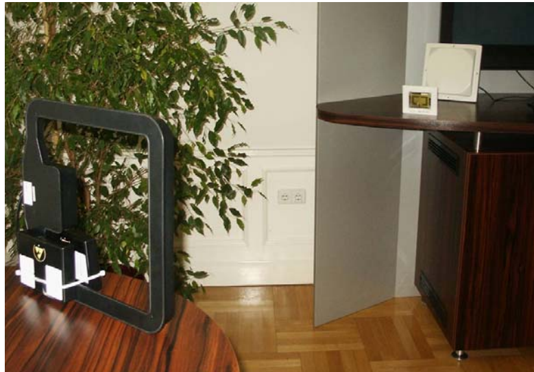
Figure 6.41: HF reader antenna (left side) and UHF reader antenna (in the background). In between the CTS transponder
