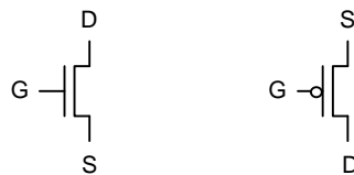
Figure 3.2: Symbol of thin oxide NMOS and PMOS transistor
