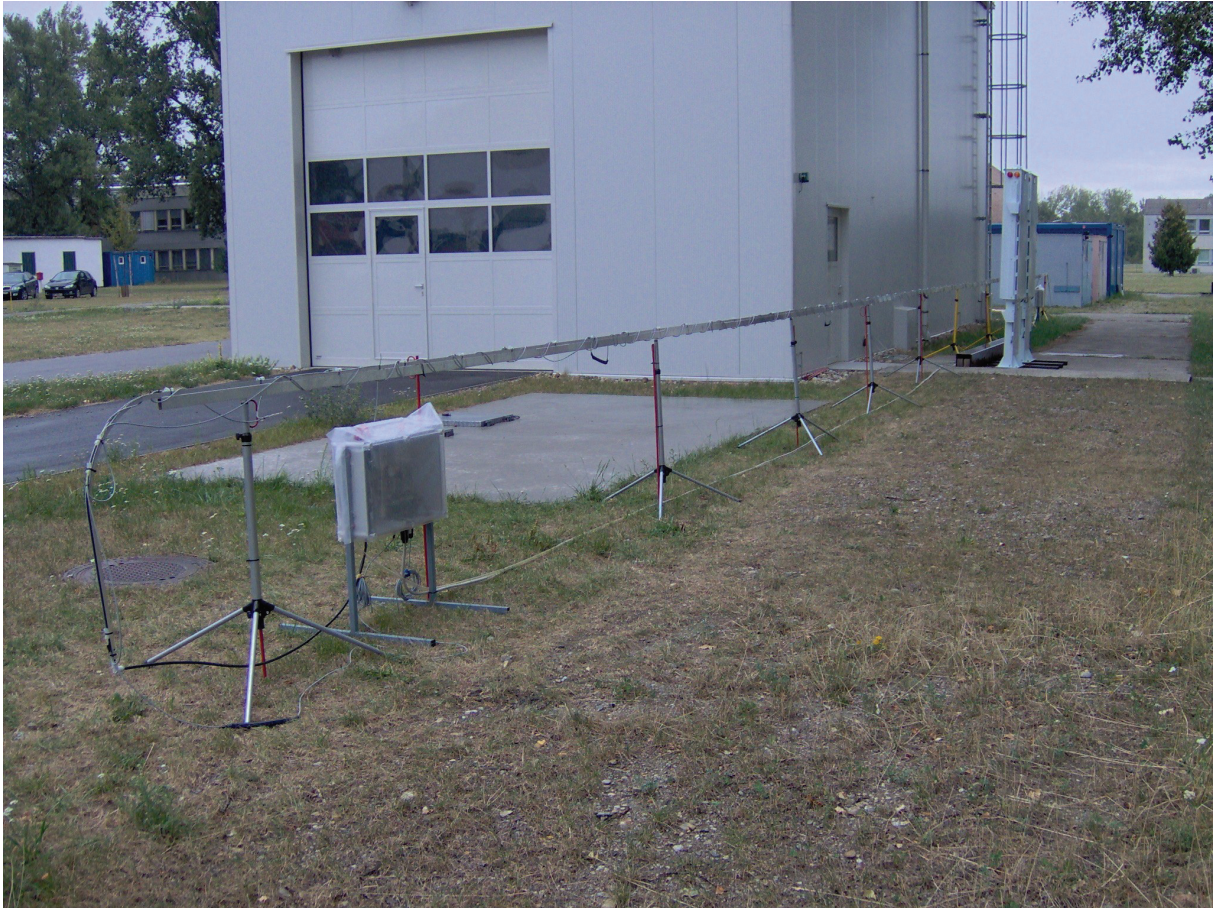
Fig. 5. Source transport system for testing of portal monitors.
