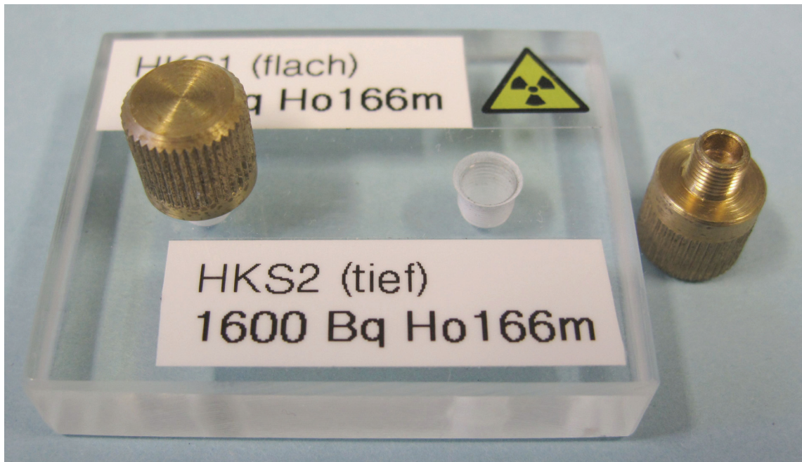
Fig. 23. Picture of the ^{166\text{m}}\text{Ho} \beta - \gamma energy calibration sources.
