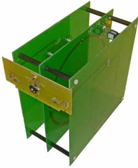
Figure 2.8: The Helmholtz arrangement according to ISO/IEC 10373-6 [Int01a].
