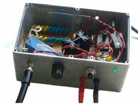
Figure 3.5: High-voltage generator that produces up to 18 kV output.
