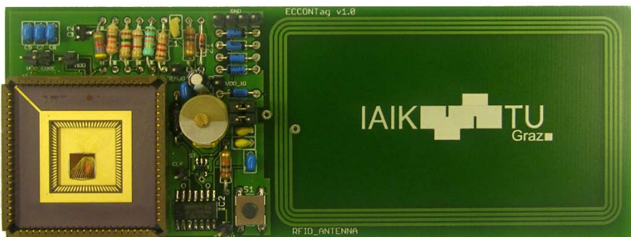
Figure 4.8: A passively powered RFID-tag prototype that is capable of generating digital signatures using ECDSA.
