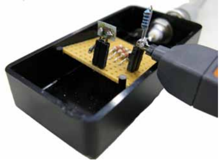
Figure 2.3: Setup for power-consumption measurements on a passive RFID tag.
