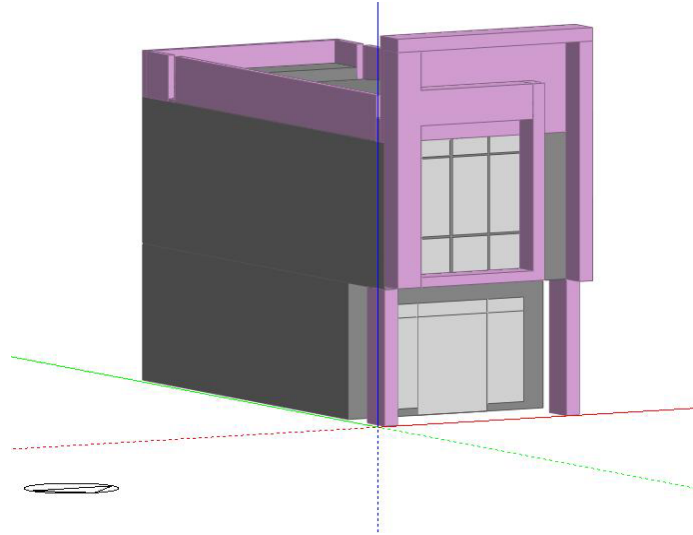
Figure 70. The Geometry of the Shophouse (generated using DesignBuilder)
