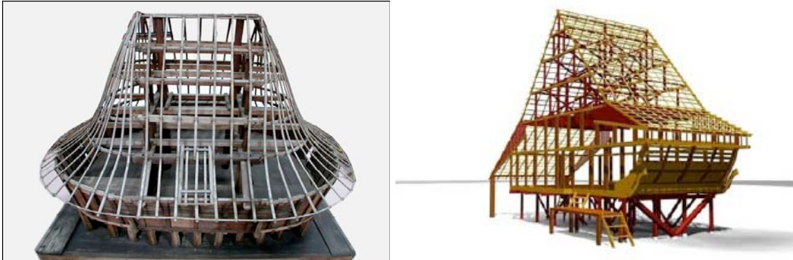
Figure 32. Three-dimensional model of a north Nias (left) and south Nias (right) house (Gruber et al. 2008)
