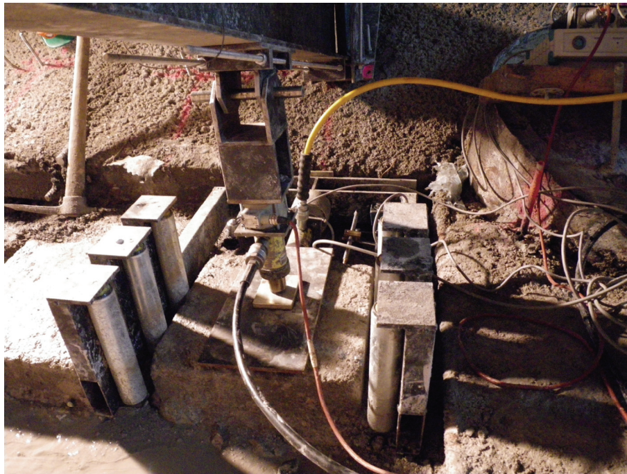
Figure 36. Detail of the alignment frame with the loading arm and LVDTs
