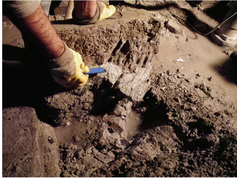
Figure 37. Failure surface formed by the structure
