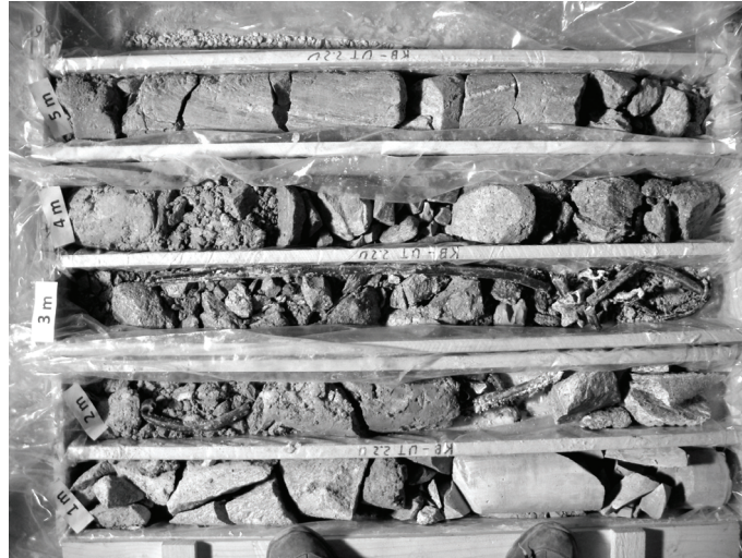
Figure 12. Core sample from a tectonic fault in the Koralm massif. Most of the fine material has been spilled out during the core drilling. Q value?
