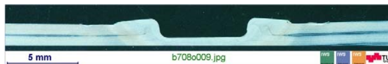
Fig. 4-62 Macrograph of friction stir spot weld in TRIP steel HCT 690 T Z100
