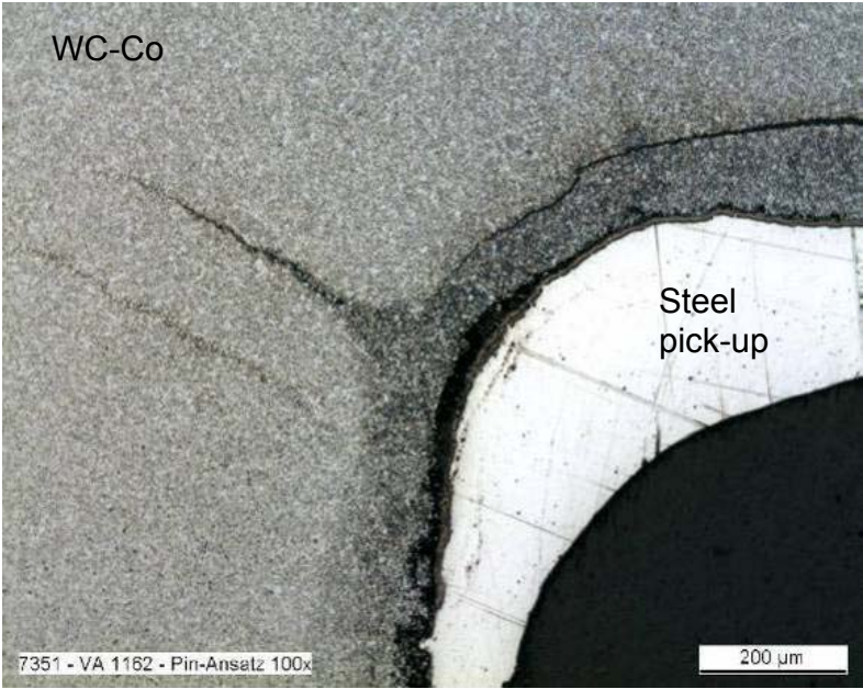
Fig. 4-72 Cracks in the probe / shoulder radii of a WC-Co tool
