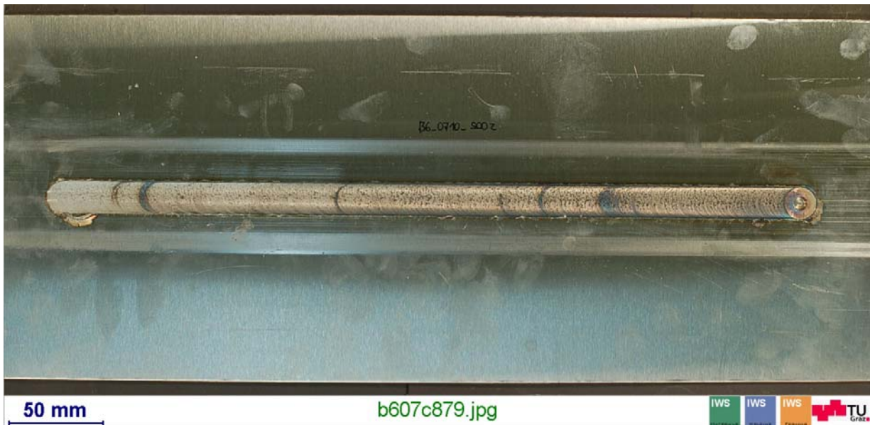
Fig. 5-10 Weld appearance of 15-5PH butt weld
