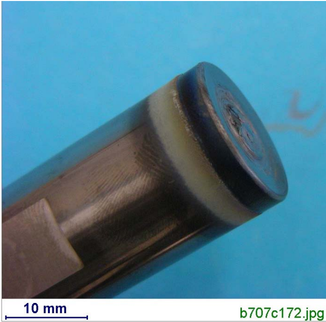
Fig. 4-73 Pin fracture of a WC-Co tool after 50mm long bead on plate welding
