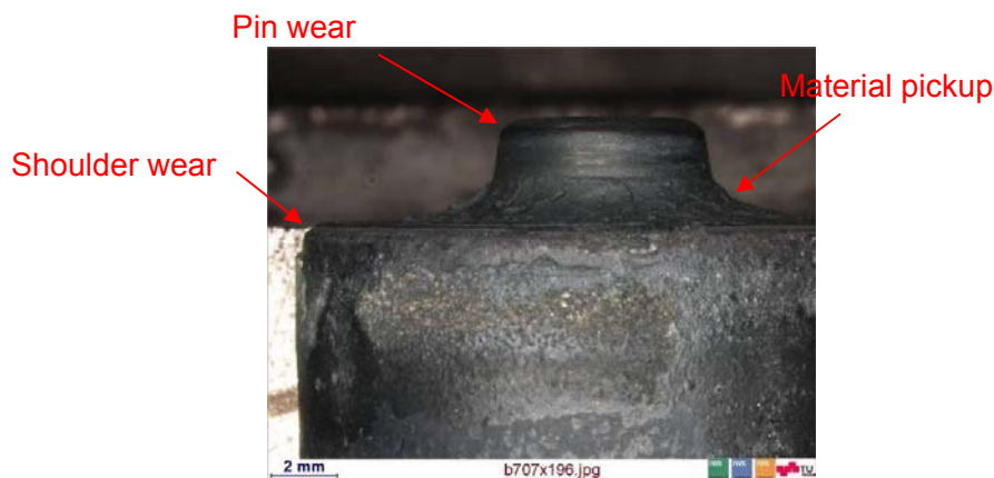
Fig. 4-27 Tool wear and material pickup after 300 mm long bead on plate welding of 4mm thick AISI304
