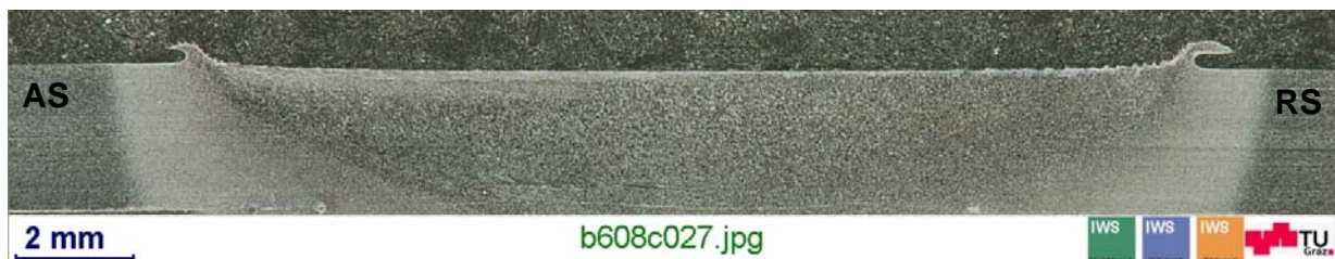
Fig. 5-12 Macrograph of transverse section of butt friction stir weld of steel 15-5PH with 1° tool tilt angle
