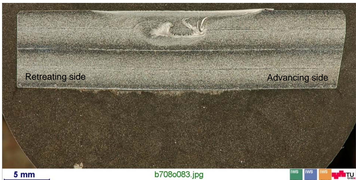
Fig. 4-35 Macrostructure of bead on plate welded steel using BB01 tool
