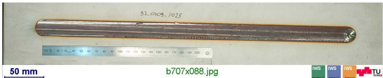
Fig. 4-34 Top surface of a 400 mm long bead on plate weld using BB01 tool
