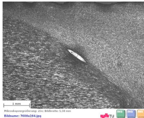
Fig. 4-53 Detail from Fig. 5-52: Copper marker at TMAZ, P002A
