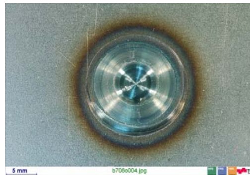
Fig. 4-61 Appearance of top surface for friction stir spot weld in TRIP steel HCT 690 T Z100
