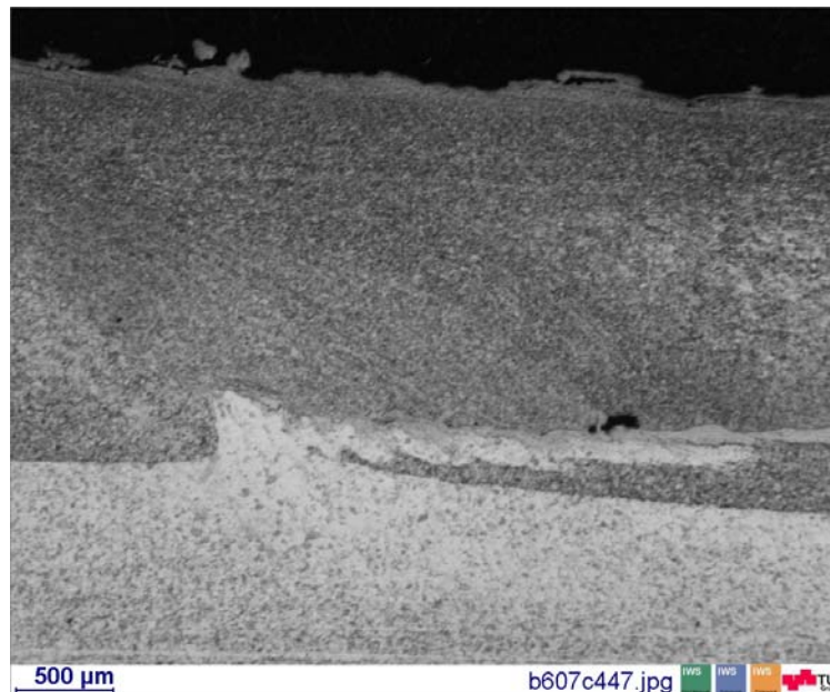
Fig. 5-8 Detail A of Fig. 5-7 showing backing plate penetration
