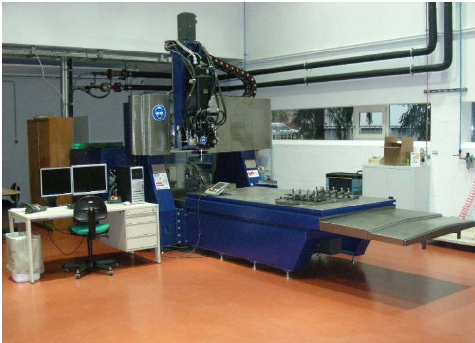
Fig. 4-9 MTS ISTIR BR4 Friction Stir Welding Machine at the Institute for Materials Science and Welding of TU Graz
