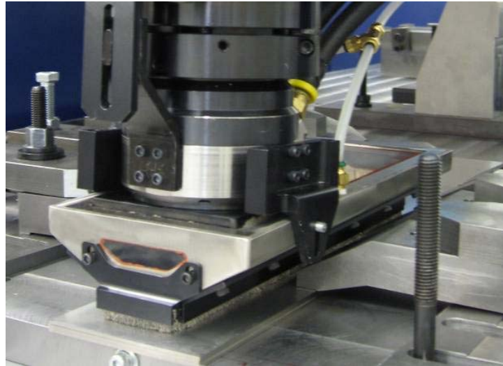
Fig. 4-13 Typical weld setup with argon shielding
