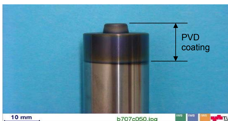
Fig. 4-37 PVD coating on probe and shoulder for a WC-Co tool
