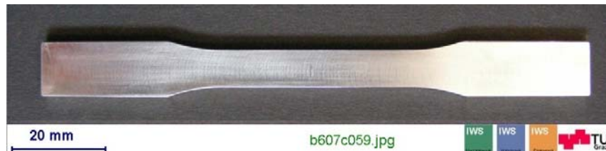
Fig. 4-18 Milled tensile sample with a thickness of 3 mm
