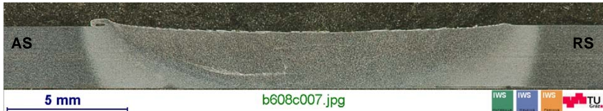
Fig. 5-19 Macrograph of transverse section of butt friction stir weld of steel 15-5PH under hardened condition
