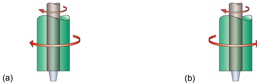
Fig. 3-4 Schematic principle of Dual-rotation FSW with equal rotation direction (a) and (b) different rotation direction [18]
