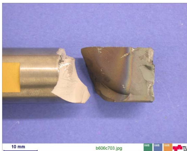
Fig. 4-32 Shaft and shoulder fracture of tool SB10
