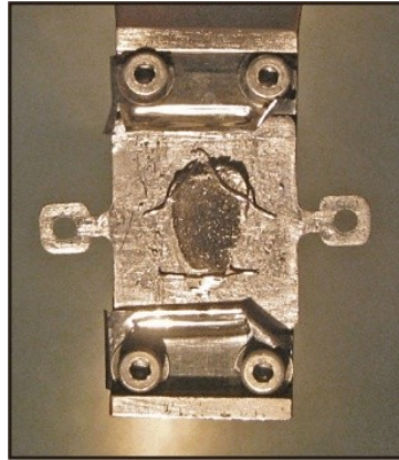
Fig. 2. 16: Photograph of the substrate, made of a palladium single crystal cleaved along the (111)-surface. The crystal is mounted to the sample holder with three tantalum-wires.
