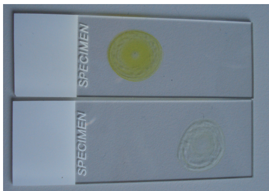
Figure 6.11: Photo of a polymer layer of polybis(-p-butylphenyl)stannane before and after heating above 150°C
