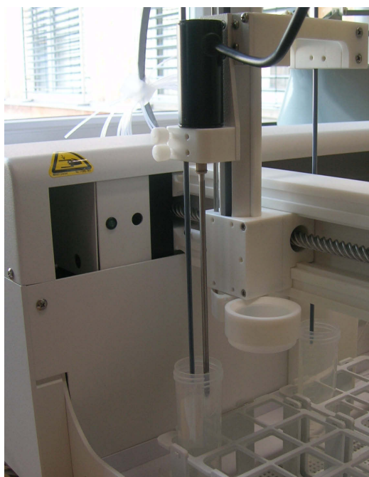
Fig. 7 - 27 Dual probe holder with stirrer and drip cup for the ASX 1400
