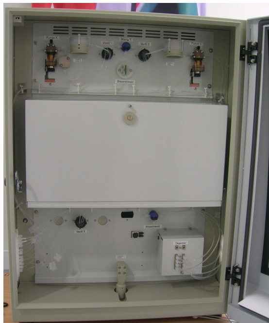
Fig. 8 - 2 Offline flow digestion system with open front door showing pumps, valves and loops
