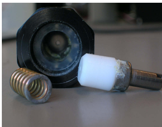
Fig. 7 - 6 Detailed Hamilton valve showing abrasion of the rotor
