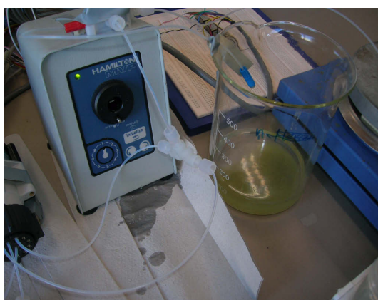
Fig. 7 - 7 Strong leakage of the Hamilton 8-port valve drive
