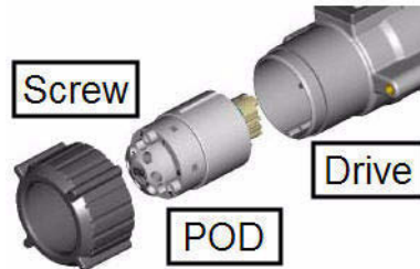
Fig. 7 - 14 Liquid end (POD), drive and quick-fix screw for the Titan HT injection valve
