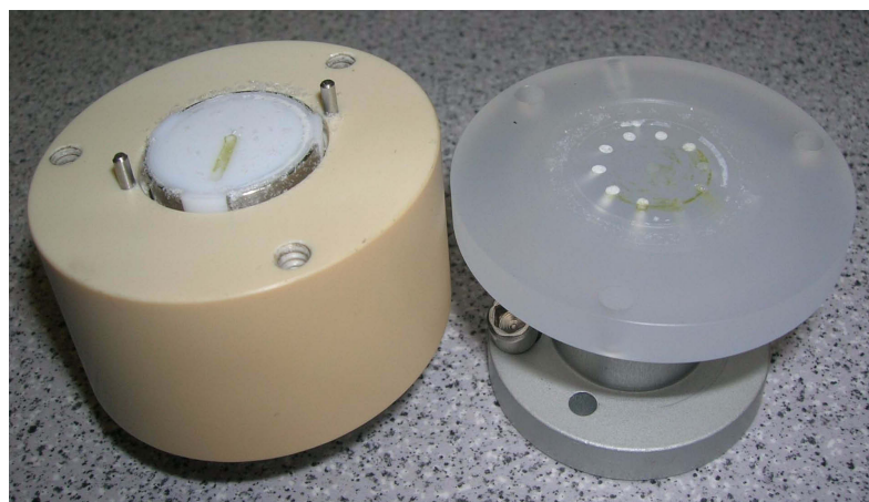
Fig. 7 - 10 Vici Cheminert rotor with spring package (left) and Kel-F stator (right)
