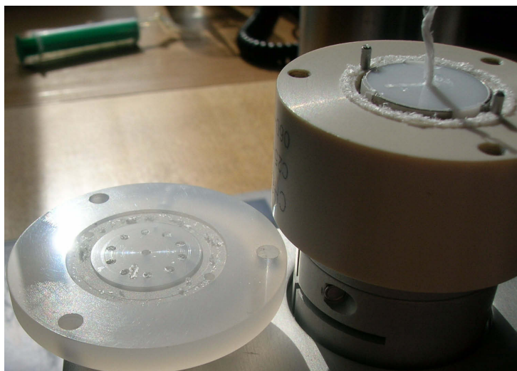
Fig. 7 - 3 Vici Cheminert Valve: massive PTFE abrasion after 170,000 dry switching experiments
