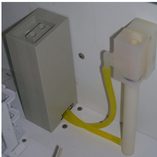
Fig. 7 - 28 Rinsing stations for the sample probe and stirrer (left) and collection probe (right)
