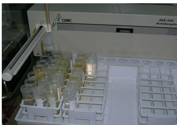
Fig. 7 - 25 Autosampler ASX 520 for single probe operation used in configuration A2
