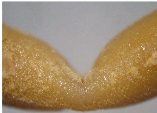
Fig. 8 - 20 Not broken used capillary made from the previous material after the bending test
