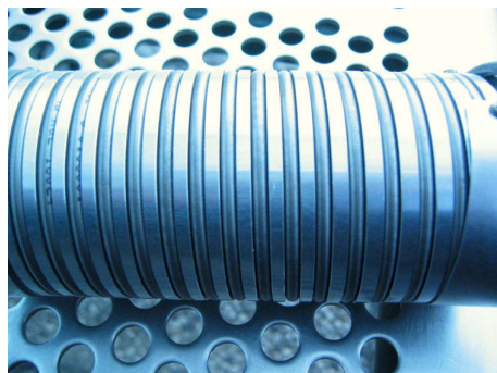
Fig. 4 - 12 Wrapped reactor tubing in an aluminum coil
