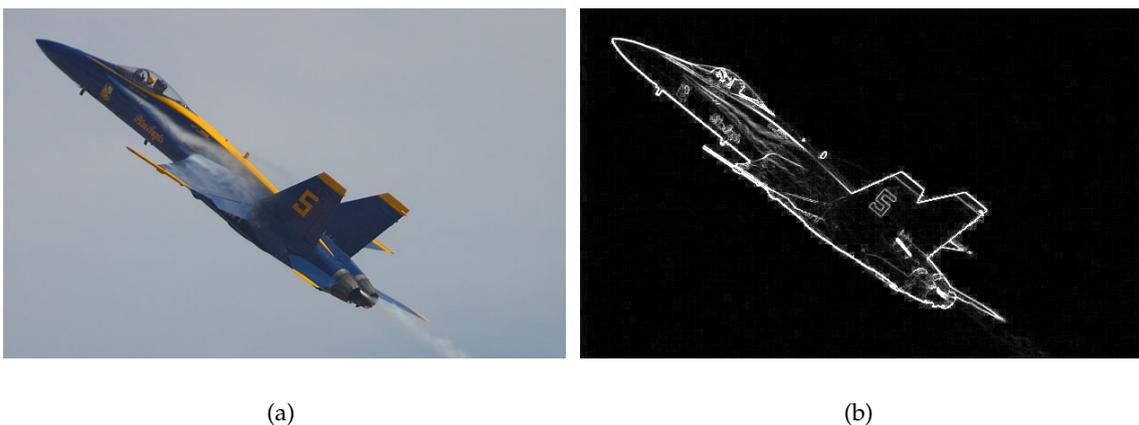
Figure 1.7: The magnitude of the image gradient shown in (b) is a powerful indicator for possible segment borders. Note that (a) was converted to grayscale before gradient computation and that the gradient was contrast enhanced for better visualization.
