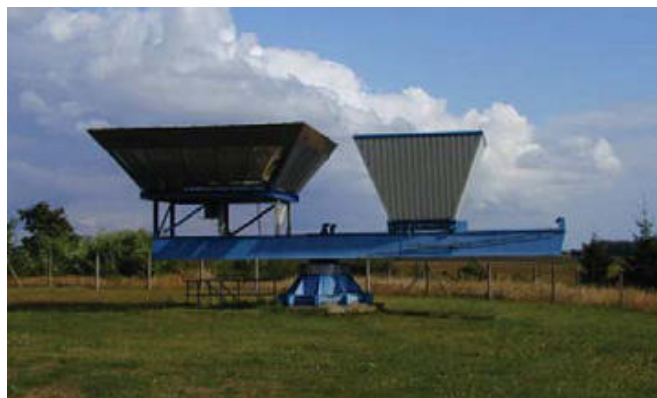
Figure 4-6: 1,290 MHz Wind Profiler Radar at Lindenberg, Germany (source: German Meteorological Service (DWD) ).
