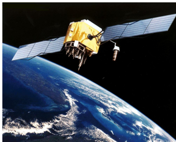
Figure 2-2: Artist impression of a GPS Block IIF satellite in orbit. (source: NASA)
