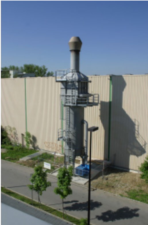
Figure 2: Picture of the 5 MW thermal air heater at the Institute for Thermal Turbomachinery and Machine Dynamics, Graz University of Technology.
