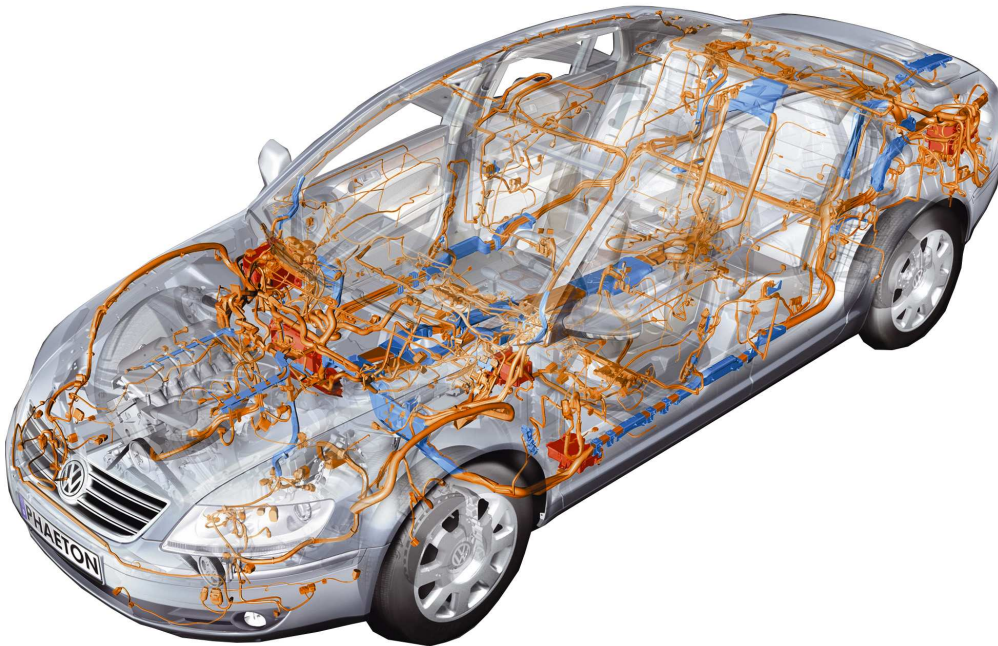
Figure 1.1: Volkswagen Phaeton: Automotive Electronics as Distributed System [6]
