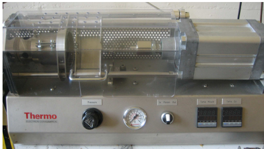
Figure 3.2-2: Injection piston (left) and steel mould (right).
