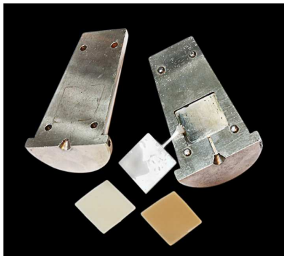
Figure 3.2-4: Compound samples produced via injection-moulding (left) and compression moulding (right).
