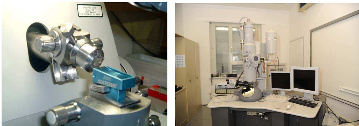
Figure 6.1-3: Microtome for ultra-thin cuts (left) and TEM (right). 82
