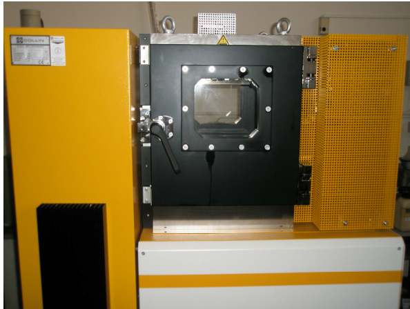
Figure 3.2-3: Collin P200PV heat-able vacuum press.
