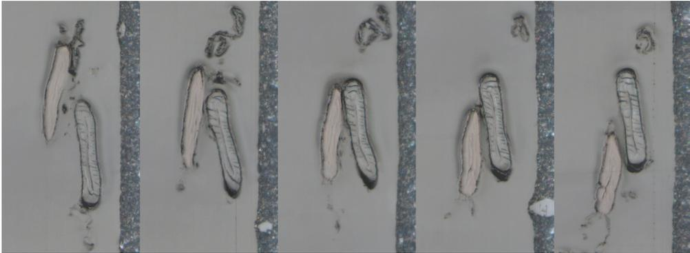
**Fig. 8.9** Microtome images explaining the deviation between measured and calculated bonded area (1)
