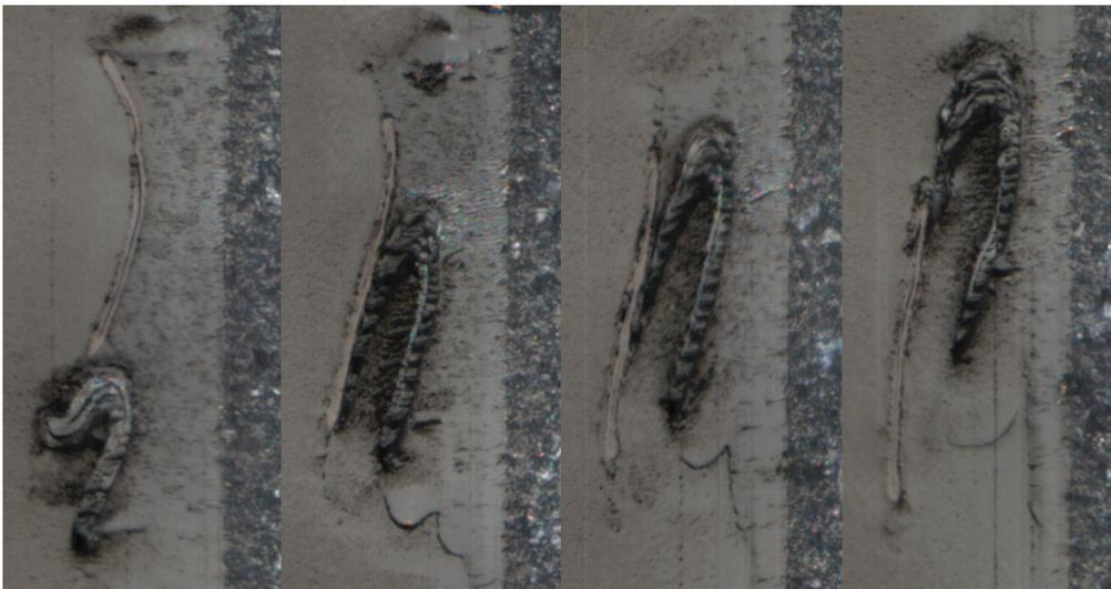
**Fig. 8.10** Microtome images explaining the deviation between measured and calculated bonded area (2)
