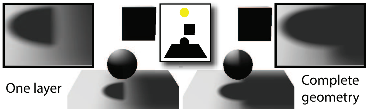
Figure 3.8: Single-sample soft shadows. The small image in the middle illustrates the scene setup consisting of a light source, a cubical occluder, a spherical occluder and a large planar receiver. Left: Incomplete shadows are computed upon using the depth of front-facing geometry only that is visible from a single point in the centre of the light source. The shadow cast by the cube incorrectly exhibits large penumbrae because the top face of the cube is incorporated only. As a result, the shadow cast by the cube onto the right hemisphere of the sphere is hardly objectionable. The shadow cast by the cube onto the plane incorrectly appears too soft. Furthermore, only the left hemisphere of the sphere is incorporated. The right hemisphere is invisible from the centre of light source. Therefore, the shadow cast by the sphere artificially appears to be cut off. This is amplified by the large penumbrae of the shadow cast by the cube. Right: The accurate shadow solution samples more layers of depth to completely capture the occluding geometry. The right hemisphere of the sphere is correctly occluded. The shadows on the plane correctly unify (image courtesy of [EASW09]).
