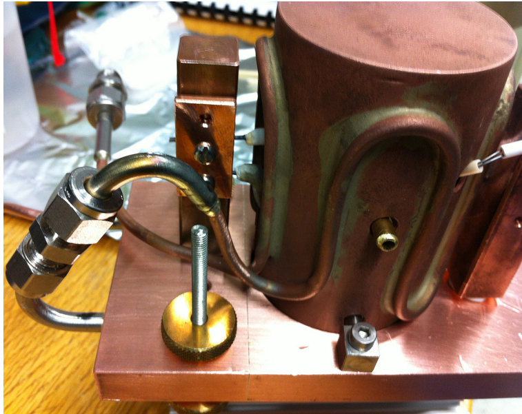
Figure 5.3.: Fully assembled gold oven with cooling shield and thermocouple. The connections for the water cooling are made of high quality steel for durability. The brass pipe to align entrance and exit holes is still in place.
