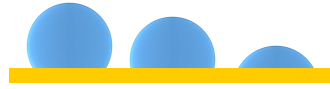
Figure 2.3.: Decreasing contact angle (from left to right) for three droplets on a solid surface.
