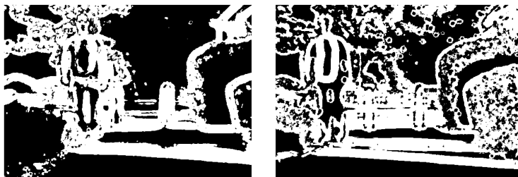
Figure 4.16: Regions of filtered informative LSS descriptors (white) on thermal (left) and optical (right) images.
