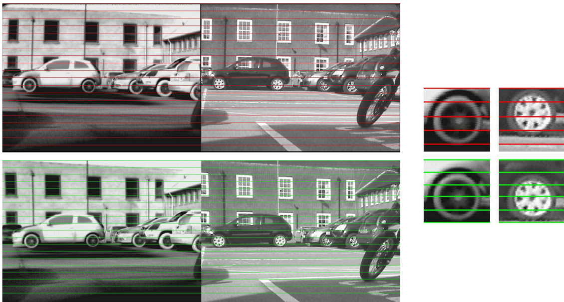
Figure 4.6: Example of a cross-spectral image pair before (top) and after (bottom) rectification.
