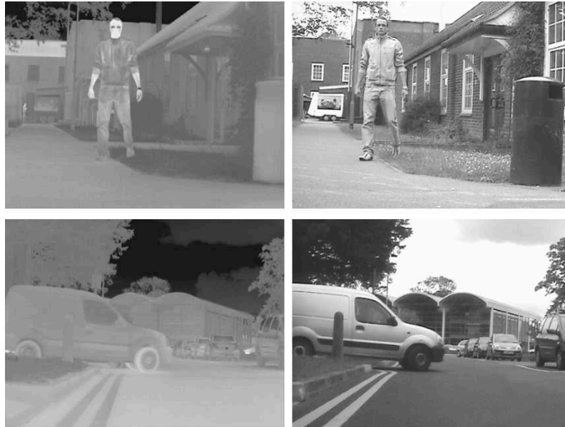
Figure 1.2: Examples of far infrared (left) and corresponding visible grayscale outdoor images (right).
