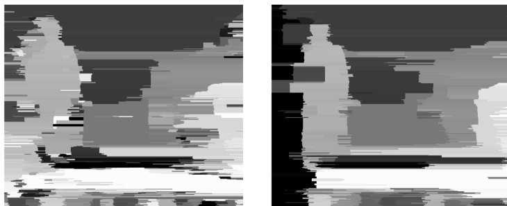
Figure 4.17: Disparity maps of SO (left) and DP (right) optimization methods using HOG matching costs.
