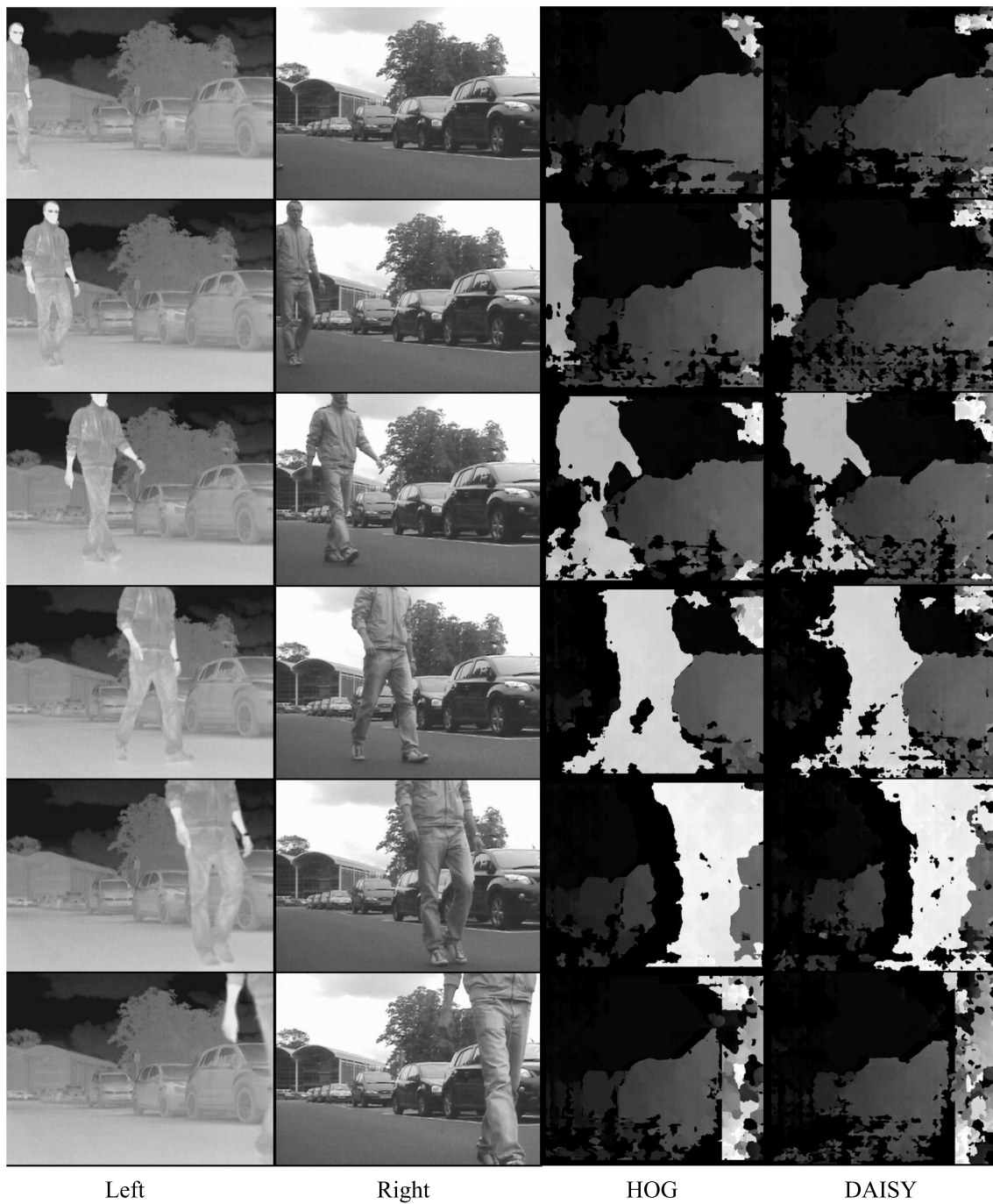
Figure 4.28: Result frames from Video 2 using HOG and DAISY matching costs with SGM.
