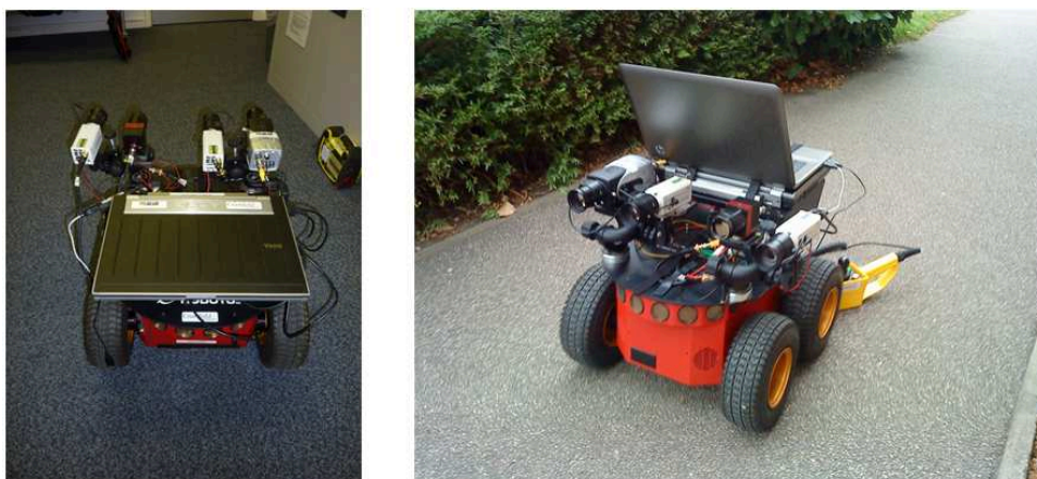
Figure 4.3: The four-camera dual stereo setup on our mobile robot.
