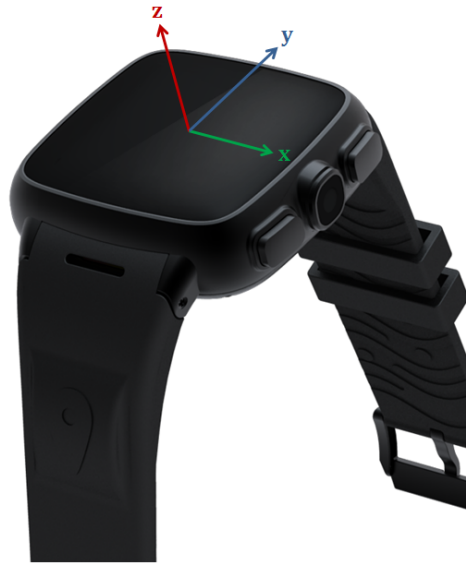
Figure 4.4: Smartwatch Omate TrueSmart with marked sensor axes.
