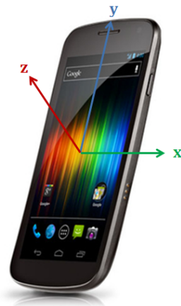
Figure 4.2: Smartphone Samsung Galaxy Nexus with marked sensor axes.
